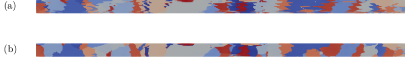
Figure 19. Stacking of successive 2D EBSD maps to reconstruct the 3D microstructure, (a) without and (b) with the use of Eq. 15
