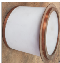
Figure 1.13: Picture of the ceramic's RF feed-through of the WEST ICRH antennas.
