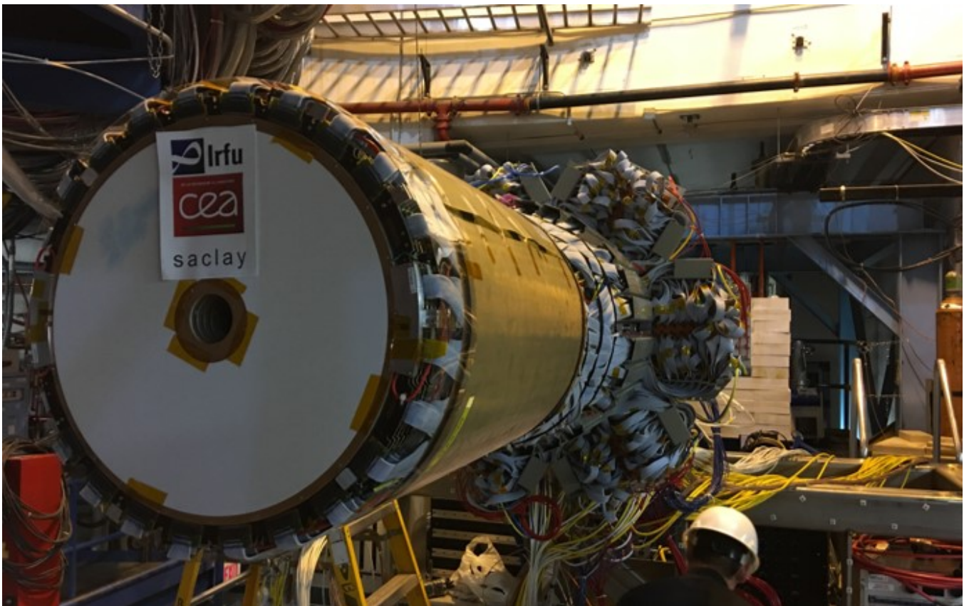
Figure 5.41: Micromegas Central Tracker and Silicon Vertex Tracker during installation at Hall B of Jefferson Laboratory in October 2017.
