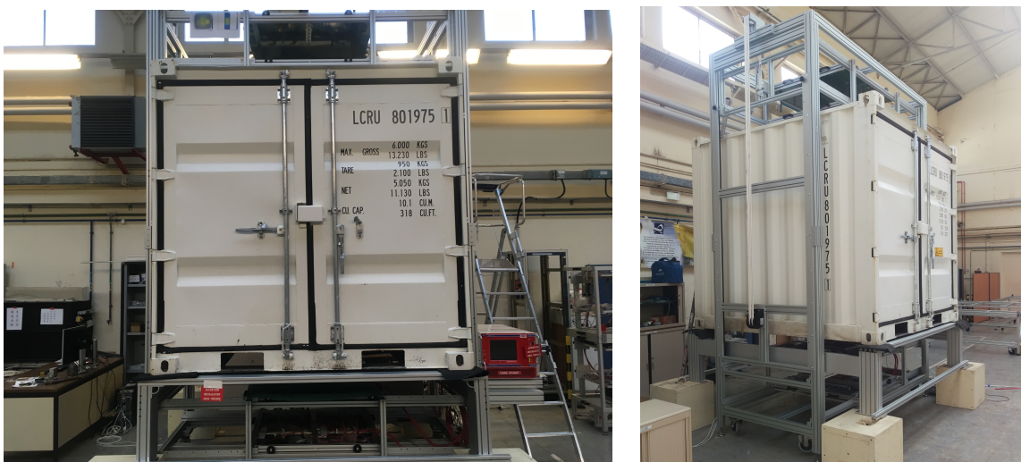
Figure 8.1: Face view [left] and side view [right] of the M-Cube muon tomography 1 m 2 scanner. The two planes below the container and the two planes above comprised 4 MultiGen each are visible.
