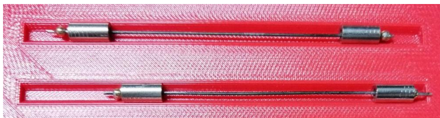
Figure II.2.3. Two IT-strands with the integrated SCUTT device.
