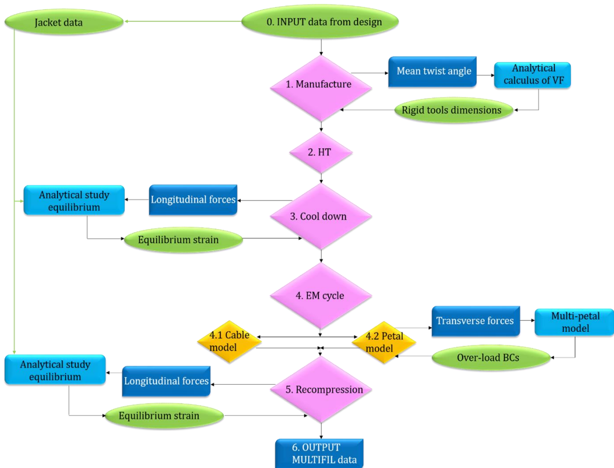
Figure III.3.1. Numerical protocol of the fusion cable simulation with MULTIFIL code.
