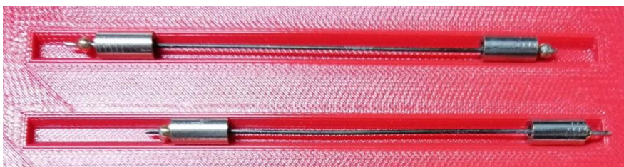
Figure II.2.3. Two IT-strands with the integrated SCUTT device.
