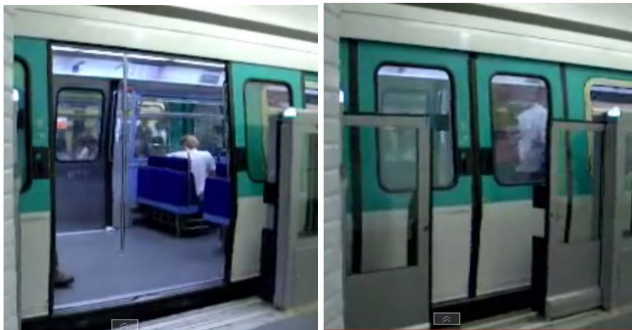
Figure 4.4 – On the left, automatic opened doors, on the right, the platform doors are automatically closing (images excerpt from YouTube)
