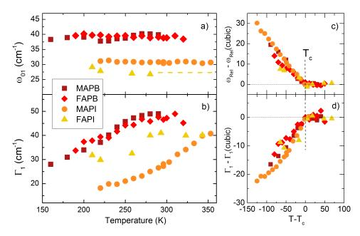
Figure 5.4: Vibrationnal parameters of the Raman mode of lowest frequency in MAPB, FAPB, MAPI, and FAPI: (a) Temperature dependence of the frequencies  $\omega_{01}$  and (b) dampings  $\Gamma_1$ . (c) Normalized relaxational frequencies  $\omega_{Rel}(\text{T-T}_C)-\omega_{Rel}(\text{cubic})$  and (d) normalized dampings  $\Gamma_1(\text{T-T}_C)-\Gamma_1(\text{cubic})$ .
