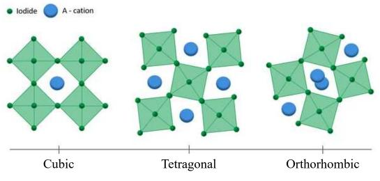
Figure 1.5: Illustration of the possible crystal structures of HOPs.
