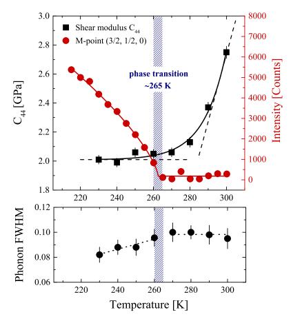
Figure 5.10: (a) Softening of  $C_{44}$  and (b) phonon width in FAPbBr<sub>3</sub> as function of temperature, between 230 and 300 K, at around the (002) Bragg reflection. Also in (a) the Bragg M point intensity (red) across a similar temperature range.
