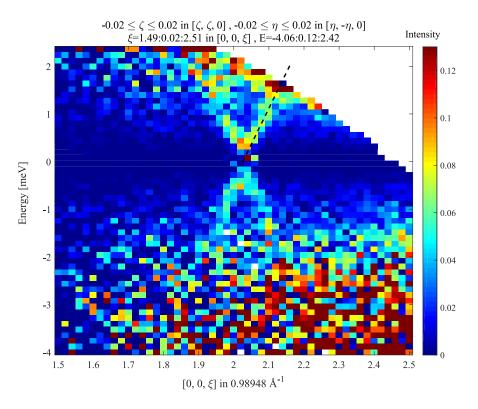
Figure B5: ToF neutron spectra measured at room temperature in MAPbI<sub>3</sub>. Longitudinal acoustic (LA) phonons around the 002 Bragg reflection are clearly seen up to energies of  $\sim 2$  meV. The slope (dashed line), corresponding to the sound velocity from the previously reported dispersion curves of the same LA phonons (Fig. 3.2), is also plotted for comparison.
