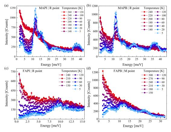
Figure 5.1: Temperature dependence of the INS optical spectra at the R point of (a) MAPI, (b) MAPB and (c) FAPI and (d) at the R point of FAPB. (a), (b) and (d) are measured at LLB on the thermal TAS (1T) and (c) on the cold TAS at LLB (4F2).
