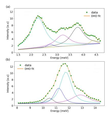
Figure B3: 1D cuts of the ToF mapping of MAPI, at Q = (002), between (a) 1.5-4.6 meV and (b) 8-14.5 meV. The data (green scatter points) is fitted (orange line) with a sum of a sum of DHOs (Eq. 2.38, section X).
