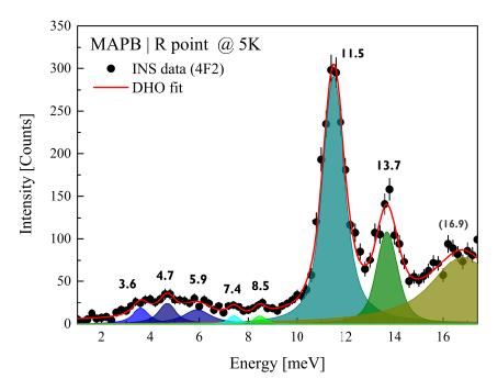
Figure B4: Optical phonon spectra, measured by TAS inelastic neutron scattering at low temperature (5 K), in MAPbBr<sub>3</sub> at the R (1/2 1/2 3/2). The experimental INS data (black scatter points) is fitted (red line) with a sum of DHOs (Eq. 2.38, section 2.2.5) and is presented with a removed background.
