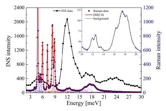
Figure 4.4: Comparison of the INS using the thermal beam instrument 1T at LLB (5 K) and Raman scattering (20 K) optical phonon spectra in MAPB, at the  $\Gamma$  point ( $\equiv (0, 0, 2)$  Bragg position for INS). Inset shows a magnification of the Raman scattering spectra in the 10-20 meV range. The energy resolution of Raman scattering is here 0.125 meV compared to the energy resolution of ~1-2 meV (over the scan energy range) for a thermal TAS.
