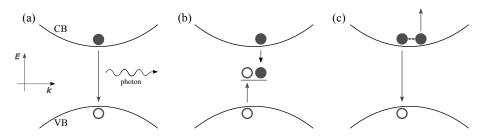
Figure 1.13: Schematic diagram of the (a) band-to-band, (b) trap-assisted and (c) Auger recombination mechanisms.
