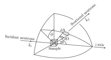
Figure 2.4: An illustration of the scattering geometry.
