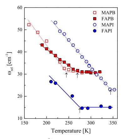
Figure B7: Relaxational frequencies  $\omega_{rel} = \omega_0^2/\Gamma$  of the lowest frequency Raman mode  $\omega_1$ , in MAPbBr<sub>3</sub>, MAPbI<sub>3</sub>, FAPbBr<sub>3</sub> and FAPbI<sub>3</sub>, as a function of temperature. The cubic-tetragonal transitions are marked (arrows), appearing to be of a less abrupt nature in Br-based samples, suggesting pre-transitional effects.
