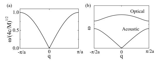
Figure 1.8: Illustration of a typical dispersion relation for a (a) monoatomic and (b) diatomic linear chains. The lower branch in (b) is the acoustic branch (same as in (a) and the upper one is the optical branch.
