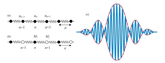
Figure 1.7: One dimension (a) monoatomic and (b) diatomic crystal lattices. The atoms are shown in their undisplaced positions, connected by a force constant C and their displacements are denoted by  $u_{n-1}$ ,  $u_n$ ,  $u_{n+1}$ . The lattice constant is a. (c) Schematic illustration of a wave packet (blue line) and the envelope of the wave packet (red dotted line). The envelope moves at the group velocity.
