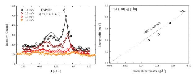
Figure B1: (a) TA phonon spectra in FAPbBr<sub>3</sub>, for different energy values around the (110) Bragg peak. To access the T2 branch, measurements were made along  $[1\bar{1}0]$  with a scattering plane of [100][010]. (b) Dispersion curve for the same phonons.
