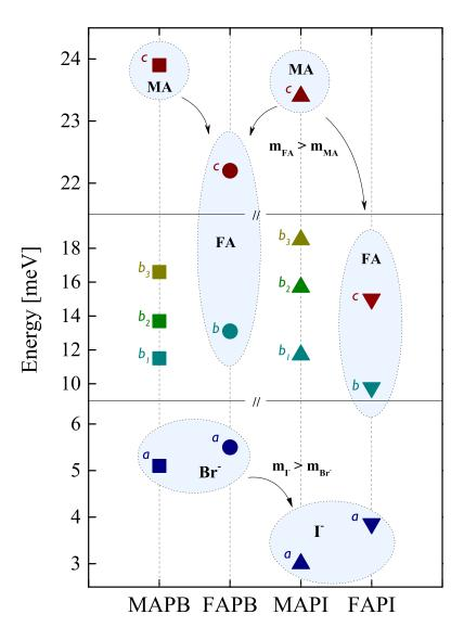
Figure 4.5: Optical phonon bundles a, b and c in MAPB, FAPB, MAPI and FAPI, illustrating the relative energy positions between compounds.
