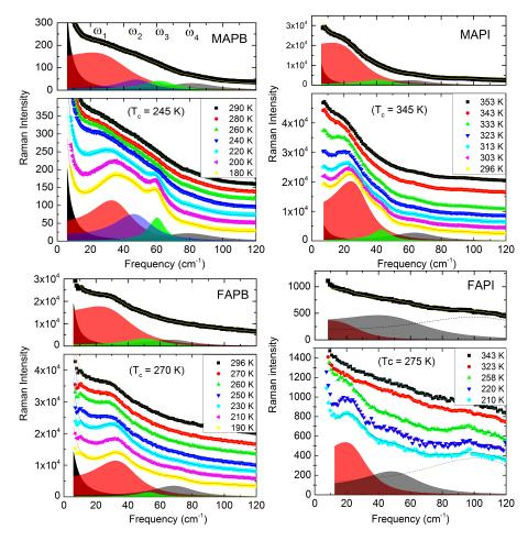
Figure 5.3: Polarized Raman spectra (symbols) in the tetragonal and cubic phases of the four HOPs, with their respective fits (plain lines). For each compound, the individual spectral line shapes  $S_i(\omega)$  (i = 1 in red, i = 2 in blue, i = 3 in green, i = 4 in gray) are shown for the lowest temperature spectra (bottom, tetragonal phase) and for the highest temperature spectra (top, cubic phase).
