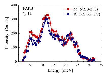
Figure B2: Optical phonon spectra, measured by TAS inelastic neutron scattering at low temperature (5 K), in FAPbBr<sub>3</sub> at the R (1/2 1/2 3/2) and M (5/2 3/2 0) Bragg points. Only a small negligible difference (in amplitude) is seen between the spectra of both points, illustrating the weak dispersion nature of the phonon modes.
