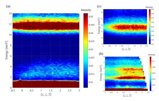
Figure 4.1: (a) Full ToF contour plot of MAPbI<sub>3</sub>, at 5 K, and zoomed in plots at (b) low (below 6 meV) and (c) high (10-14 meV) energy range.
