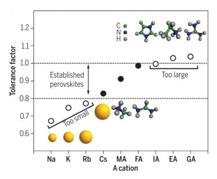
Figure 1.4: Tolerance factor of APbI<sub>3</sub> perovskite with A cations that are too small (Na, K, Rb), established (Cs, MA, FA), or too large [imidazolium (IA), ethylamine (EA), guanidinium (GA)]. The inset images depict the cation structures. Empirically, perovskites with a tolerance factor between 0.8 and 1.0 (dotted lines) show a photoactive black phase (solid circles) as opposed to nonphotoactive phases (open circles). Reprinted from [1].
