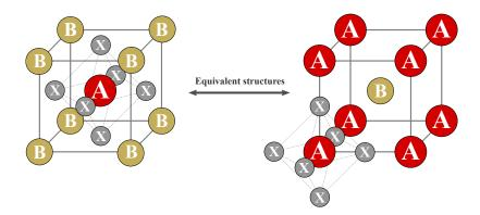
Figure 1.3: A generic perovskite crystal structure of the form ABX<sub>3</sub>. Note that the two structures are equivalent – the left-hand structure is drawn so that atom B is at the (0, 0, 0) position while the right-hand structure is drawn so that atom (or molecule) A is at the (0, 0, 0) position. Also note that the lines are a guide to represent crystal orientation rather than bonding patterns.
