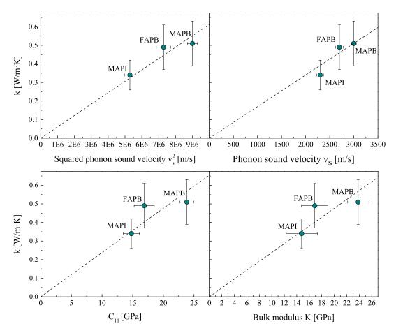
Figure 3.5: Thermal conductivity  $\kappa$  as a function of (a) longitudinal phonon sound speed  $\mathbf{v}_{LA}$ , (b)  $\mathbf{v}_{LA}^2$ , (c)  $C_{11}$  and (d) bulk modulus K. The dashed line is a linear fit intercepting at y = 0.
