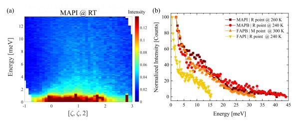
Figure 5.2: (a) ToF contour plot of MAPI at RT, for an energy range of 0-13 meV. (b) Normalized TAS spectra of optical phonons at the M (5/2, 1/2, 0) and R (1/2, 1/2, 3/2) points of the BZ, in MAPB, MAPI, FAPB and FAPI. The temperature of each scan is labelled.
