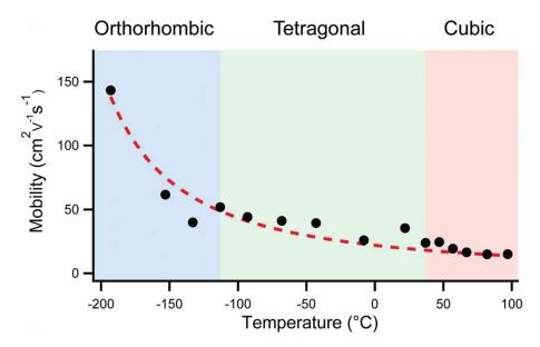
Figure 1.14: Mobility in MAPbI<sub>3</sub> as a function of temperature, determined from optical-pump–THz probe measurements. The black dots represent data, and the dashed line is the theoretical  $T^{-3/2}$  dependence predicted for band-like transport. Reprinted from [8].
