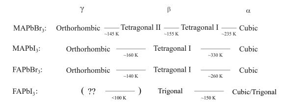
Figure 1.6: Simplified overview of the structural phases adopted at different temperatures by MAPbBr<sub>3</sub>, MAPbI<sub>3</sub>, FAPbBr<sub>3</sub> and FAPbI<sub>3</sub>.
