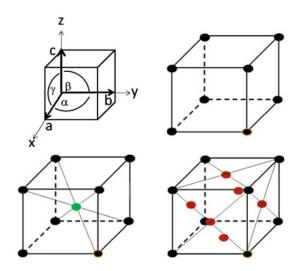
Figure A1: (a) The three basic vectors  $\boldsymbol{a}$ ,  $\boldsymbol{b}$  and  $\boldsymbol{c}$  and the angles between a pair of vectors,  $\alpha$ ,  $\beta$ , and  $\gamma$ . Three lattices of the cubic system, namely the (b) simple cubic, (c) face-centered cubic (FCC) and (d) body-centered cubic (BCC).
