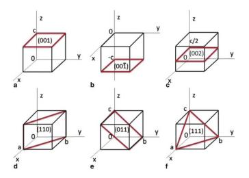
Figure A2: Various planes in a cubic lattice: (a) The (001) plane; (b)  $(00\overline{1})$  plane; (c) (002) plane; (d) (110) plane; (e) (011) plane and (f) (111) plane.
