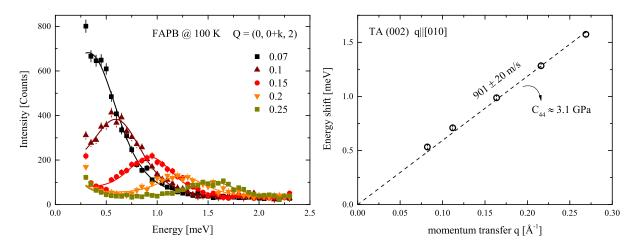
Figure B8: (a) TA phonon spectra in FAPbBr<sub>3</sub> at 100 K, for different Q positions going away from the (002) Bragg peak, along the [010]. (b) Dispersion curve for the same phonons.
