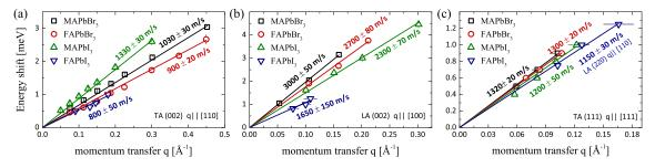
Figure 3.2: Acoustic phonon dispersion curves for the four HOPs, as measured by INS. (a) TA and (b) LA phonons at (002); (c) TA phonons at (111) in MAPB, MAPI and FAPB and LA phonons at (220) in FAPI.
