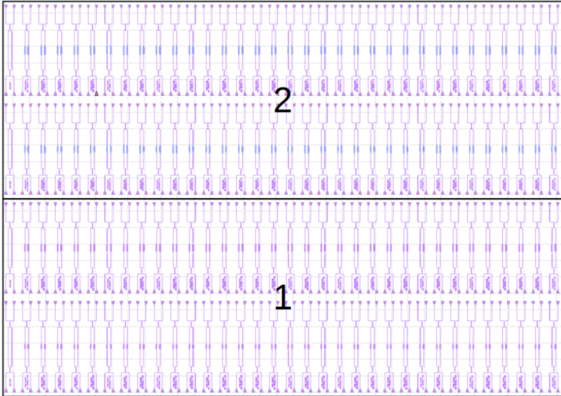
Figure C.4 – Subcell for SWG interdigitated combs waveguides within Mach-Zehnder interferometers.
