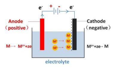
Figure 2-1 Schematic of electrodeposition
