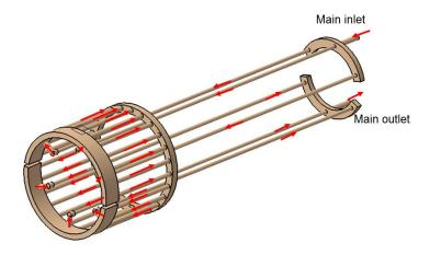
Figure 3-7 Water cooling loop design of the RF contact holder
