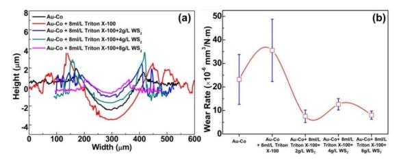
Figure 5-33 2-D profiles of wear tracks and wear rates of different coatings
