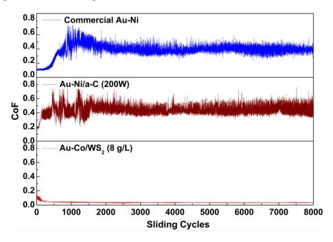
Figure 5-36 CoF of different coatings in N2 atmosphere
