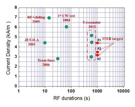
Figure 1-5 Summary of Multi-Contact LA-CUT RF experiment results in CEA
