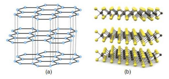
Figure 2-15 Crystal structure of: (a). graphite and (b). MoS<sub>2</sub> [78, 79]
