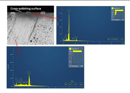
Figure 3: SEM and EDS results of cross-polished sample
