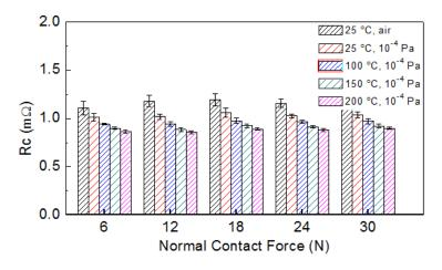
Figure 4-37 Rc measurement results of the Ag on CuCrZr/Rh on 316L pair under different contact force and temperature
