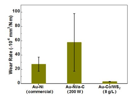
Figure 5-37 Wear rate of different coatings in N<sub>2</sub> atmosphere
