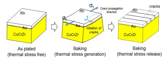
Figure 4-14 Failure mechanism of the Rh coating during baking
