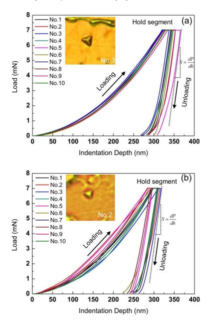
Figure 4-6 Nanoindentation load—displacement curves of Au-Ni coatings: (a) original coating, (b) thermally aged coating
