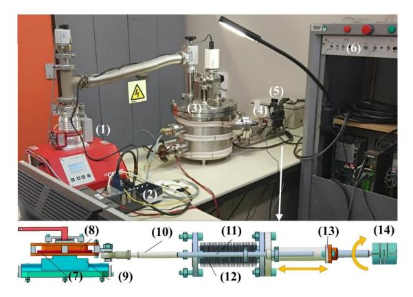
Figure 2-22 A photograph of the HV-MTEST assembly: (1). High vacuum pumping set; (2). NI cRIO-9002; (3). Vacuum tank with heaters; (4). Motor drive system; (5). Temperature regulator; (6). Motor controlling system; (7). Sample heater; (8). Sample holder plate; (9). Ball linear guide; (10). Central shaft; (11). Guide rods; (12). Bellows; (13). Screw nut mechanism; (14). Flexible coupling.
