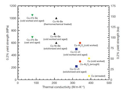
Figure 3-4 Yield stresses and thermal conductivities of copper alloys [112]
