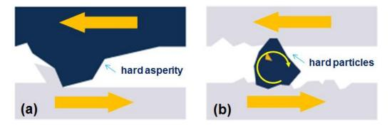
Figure 2-14 Illustration of two-body (a) and three-body (b) abrasive wear [72]
