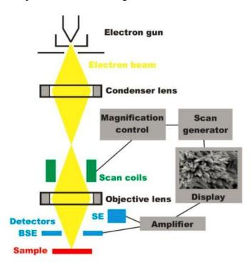
Figure 2-4 Schematic diagram of SEM system [37]
