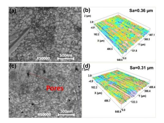
Figure 4-4 Observation results of surface morphology of coating surfaces: (a) SEM image of the surface of the original coating, (b) 3D interferometric image of the surface of the original coating, (c) SEM image of the surface of the thermally aged coating, (d) 3D interferometric image of the surface of the thermally aged coating
