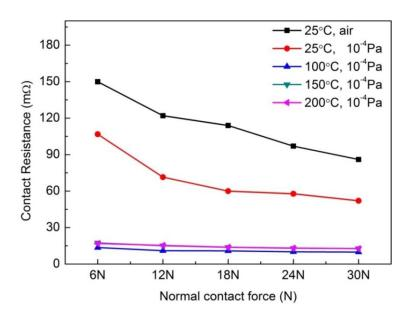
Figure 4-27 Rc measurement results of the CuCrZr/ 316L pair under different contact force and temperature
