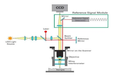
Figure 2-3 Schematic of a 3D optical profiler [35]
