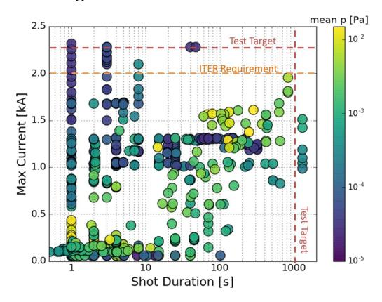
Figure 3-12 Maximum current achieved on the contact under test versus the total shot duration in seconds (in log scale). The marker colour corresponds to the average pressure during (and a few seconds after) the shot [127]
