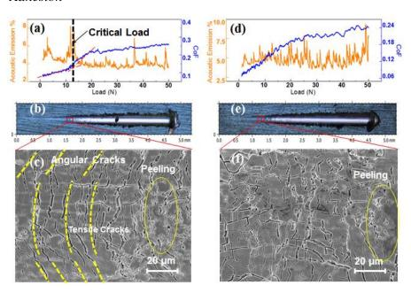
Figure 4-18 Scratch tests results of Rh coating on CuCrZr substrates: (a, d) Acoustic emission and CoF signals of original and thermally aged samples, (b, e) Optical microscope images of scratch tracks of original and thermally aged samples, (c, f) SEM micrographs of cracks on the scratch tracks of original and thermally aged samples
