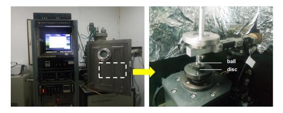
Figure 2-17 High vacuum tribometer
