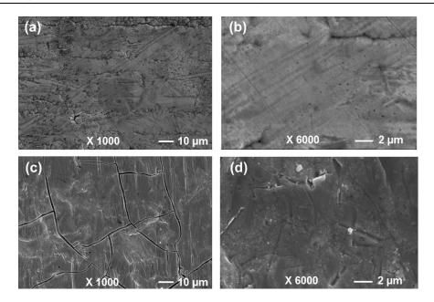
Figure 4-23 SEM images of Au-Ni (on CuCrZr) surface and Rh (on 316L) surface: (a) Au-Ni surface ×1,000, (b) Au-Ni surface ×10,000, (c) Rh surface ×1,000, (d) Rh surface ×10,000
