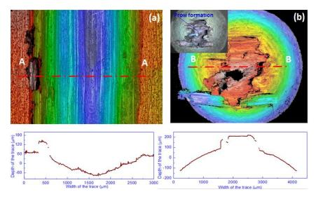
Figure 4-35 3D morphologies and depth profiles of the worn samples: (a) Rh on CuCrZr plate sample, (b) Au-Ni on CuCrZr pin sample
