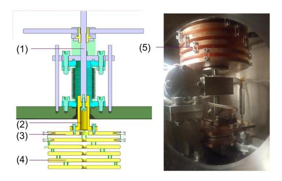
Figure 2-21 Loading system of the HV-MTEST: (1). Load lifting mechanism; (2).  $Al_2O_3$  insulation joint; (3). Dead load support; (4). Dead load plates  $(6N \times 5)$ ; (5). Hocks  $(\times 16)$
