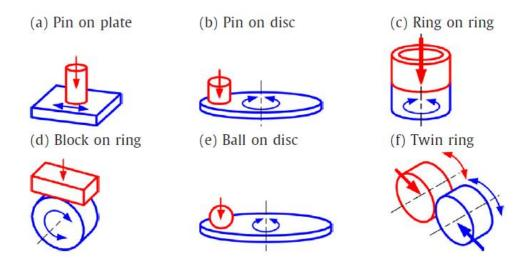
Figure 2-16 Main configurations of tribometers [92]
