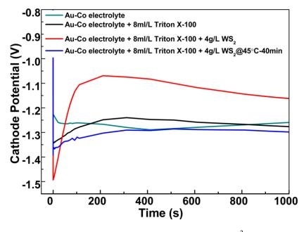
Figure 5-23 The potential-time (E-t) curves obtained at  $J=5~A/dm^2$  from the electrolyte of Au-Co and Au-Co with Triton X-100 and WS<sub>2</sub> particles.
