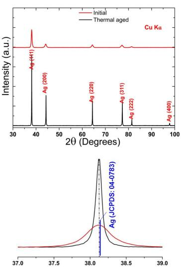
Figure 4-11 XRD pattern of Ag-Sb coating on CuCrZr (original and thermally aged)
