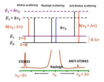
Figure 2-9 Energy level diagram for Raman scattering
