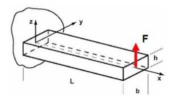
Figure 2-28 Sketch of the cantilever beam with force load
