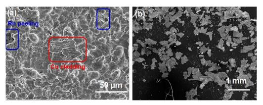
Figure 4-33 SEM images of wear track and wear debris: (a) wear track of Rh on 316L, (b) wear debris
