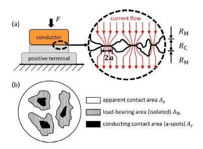
Figure 2-10 Schematic of current constriction and real contact area [56]
