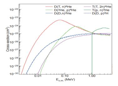
Figure 1-1 Effective cross sections of major fusion reactions [2]
