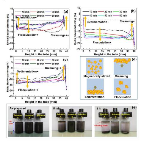
Figure 5-20 Results of  $WS_2$  particle stability measurements: (a).  $\Delta BS\%$  profiles of electrolyte A shown in Table 5-2, (b).  $\Delta BS\%$  profiles of electrolyte B, (c).  $\Delta BS\%$  profiles of electrolyte C (d). Schematic of  $WS_2$  particle behavior in electrolytes, (e). Evolution of the three electrolytes according to the waiting time
