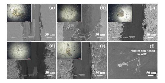
Figure 5-32 Worn surface morphologies of different coatings and their counterpart balls: (a). Au-Co, (b). Au-Co with 8 ml/L Triton X-100, (c). Au-Co with 8 ml/L Triton X-100 and 2 g/L WS<sub>2</sub>, (d). Au-Co with 8 ml/L Triton X-100 and 4 g/L WS<sub>2</sub>, (e). Au-Co with 8 ml/L Triton X-100 and 8 g/L WS<sub>2</sub>, (f). Transfer film of Au and WS2 on the worn surface of the ball shown in (c)
