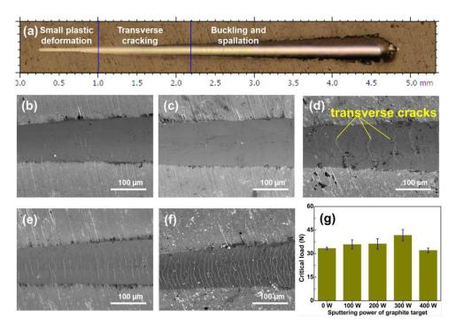
Figure 5-8 Scratch test results: (a). Optical microscope image of the full scratch track on the 400 W sample, (b-f). SEM images of scratch tracks from 0 W to 400 W, (g). Critical loads of coatings
