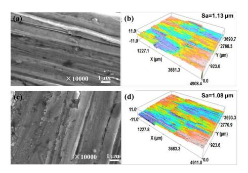
Figure 4-10 Coating surface morphology: (a, b) SEM image and 3D interferometric image of the original coating surface, (c, d) SEM image and 3D interferometric image of the thermally aged coating
