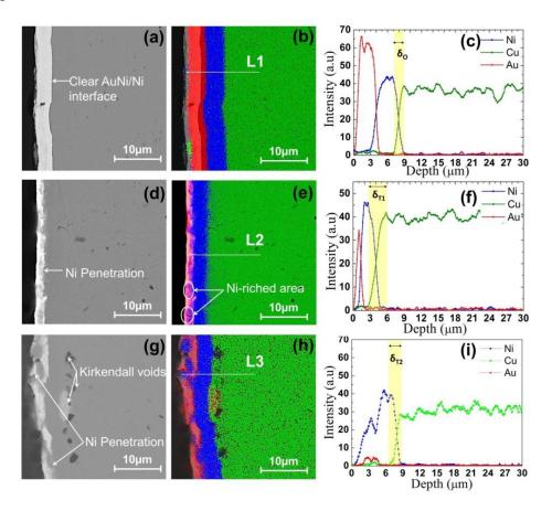
Figure 4-7 Results of SEM-EDS mapping and line scan at coating interfaces: (a, d, g) SEM images of original coating, thermally aged coating at position 1 and thermally aged coating at position 2; (b, e, h) EDS mapping images of original coating, thermally aged coating at position 1 and thermally aged coating at position 2; (c, f, i) element profiles along lines 1, 2 and 3
