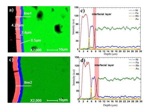
Figure 4-21 Mapping and depth profile of the Rh coating on 316L substrate: (a) EDS mapping of original sample section, (b) Elements profiles along line1, (c) EDS mapping of thermally aged sample section, (d). Elements profiles along line2
