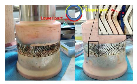
Figure 3-16 RF contact holder and RF contact after RF tests<sup>2</sup>
