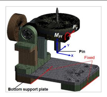
Figure 2-23 FEM and meshing of the HV-MTEST
