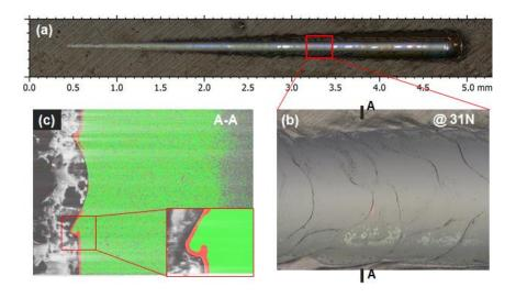
Figure 5-17 Adhesion performance of Ni (3 A/dm<sup>2</sup>): (a). Scratch track, (b). Details picture of the first delamination area, (c). EDS mapping of the A-A cross-section
