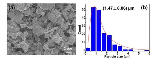
Figure 5-19 SEM and particle size (diameter) distribution of WS<sub>2</sub> after sonication
