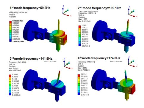
Figure 2-27 Deformation of each mode of natural vibration
