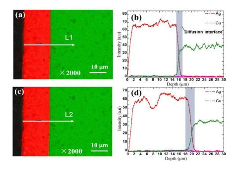
Figure 4-12 Results of SEM-EDS mapping and line scan at coating interfaces: (a,c) EDS mapping images of the original coating and the thermally aged coating, (b, d) Element profiles along lines 1 and 2
