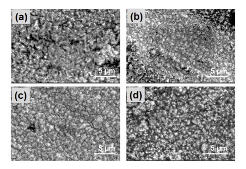
Figure 5-14 SEM images of Ni coatings plated under different current densities: (a). 2 A/dm<sup>2</sup>, (b). 3 A/dm<sup>2</sup>, (c). 4 A/dm<sup>2</sup>, (d). 5 A/dm<sup>2</sup>
