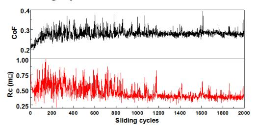
Figure 4-31 Evolution of the Rc and CoF for the Au-Ni on CuCrZr/ Rh on 316L pair under 2000 cycles of sliding test at Fn=18 N, 1 mm/s, 200 °C, 1.5×10<sup>-3</sup> Pa
