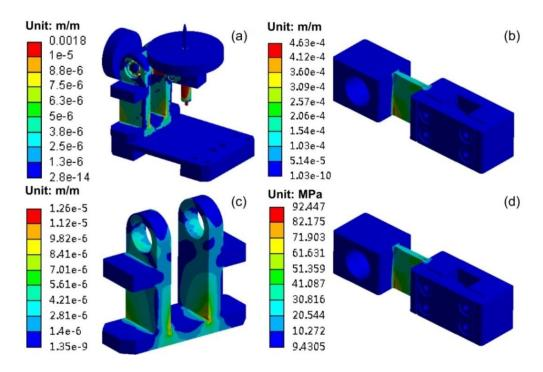
Figure 2-24 Structural analysis results under Ff=60 N: (a). global strain distribution; (b). strain distribution on the cantilever beam; (c). strain distribution on the support; (d). stress distribution on the cantilever beam.
