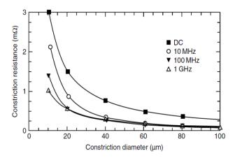
Figure 2-11 Dependence of constriction resistance on constriction diameter for current frequencies ranging from DC to 1 GHz AC [59]
