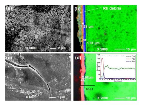
Figure 4-24 SEM and EDS mapping of Au-Ni (on CuCrZr) and Rh (on CuCrZr): (a) SEM image of Au-Ni surface, (b) EDS mapping of Au-Ni cross-sectional surface, (c) SEM image of Rh surface, (d) EDS mapping of Rh cross-sectional surface
