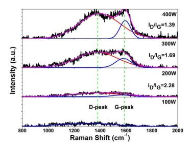
Figure 5-5 Raman spectra of the Au-Ni/a-C composite coating under different sputtering powers of the graphite target
