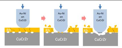
Figure 4-36 Wear mechanisms of Au-Ni on CuCrZr vs. Rh on CuCrZr pair
