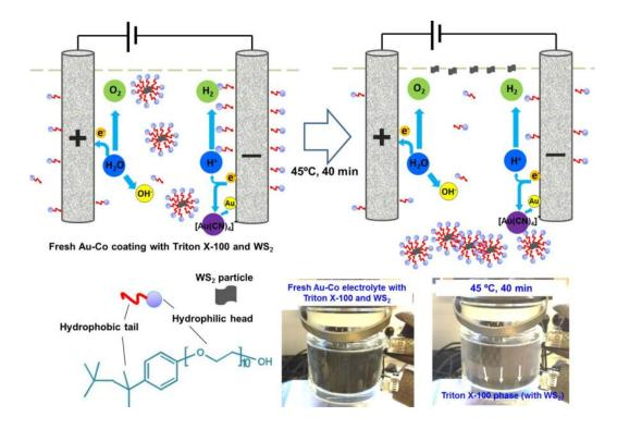
Figure 5-24 Schematic illustration of Triton X-100 surfactant assembly on WS<sub>2</sub> particles
