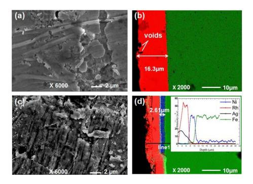
Figure 4-25 SEM and EDS mapping of Ag-Sb (on CuCrZr) and Rh (on 316L): (a) SEM image of Ag-Sb surface, (b) EDS mapping of Ag-Sb cross-sectional surface, (c) SEM image of Rh surface, (d) EDS mapping of Rh cross-sectional surface
