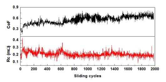
Figure 4-40 Evolution of the Rc and CoF for the Ag on CuCrZr/Rh on CuCrZr pair under 2000 cycles of sliding test at Fn=18 N, 1 mm/s, 200 °C,  $1.4\times10^{-3}$  Pa
