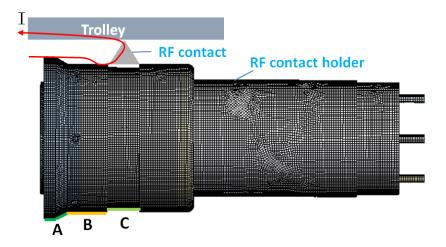
Figure 3-10 RF contact holder thermal analysis model
