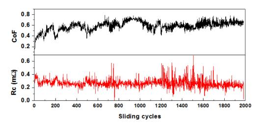
Figure 4-34 Evolution of the Rc and CoF for the Au-Ni on CuCrZr/ Rh on CuCrZr pair under 2000 cycles of sliding test at Fn=18 N, 1 mm/s, 200 °C, 9.9×10<sup>-4</sup> Pa
