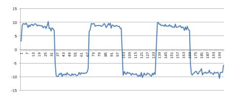
Figure 1. HV-MTEST strain output signal with slight wear
