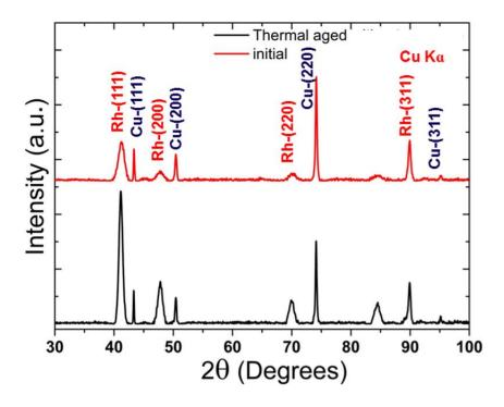
Figure 4-15 XRD patterns of Rh coatings on CuCrZr substrates (original and thermally aged)
