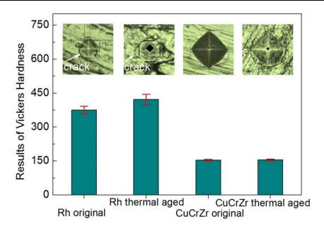
Figure 4-16 Measurement of Vickers hardness of Rh coating and CuCrZr substrate
