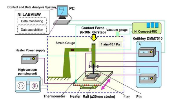
Figure 2-18 Scheme of the HV-MTEST facility
