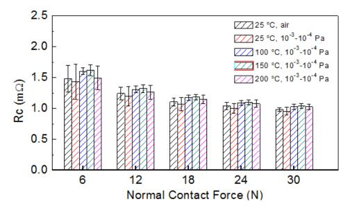
Figure 4-30 Rc measurement results of the Au-Ni on CuCrZr/Rh on 316L pair under different contact force, temperature and atmosphere conditions
