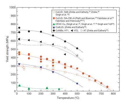
Figure 3-3 Yield stresses of copper alloys under different temperature [112]
