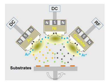
Figure 2-2 Schematic configuration of the magnetron sputtering system
