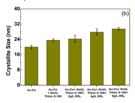
Figure 5-30 Crystallite size calculated from Au-Co (111) peaks
