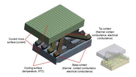
Figure 3-19 Thermal analysis model of LA-CUT RF contact
