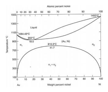
Figure 3 Au-Ni binary alloy phase diagram
