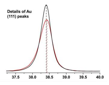
Figure 4-5 XRD pattern of Au-Ni coating on CuCrZr (original and thermally aged)
