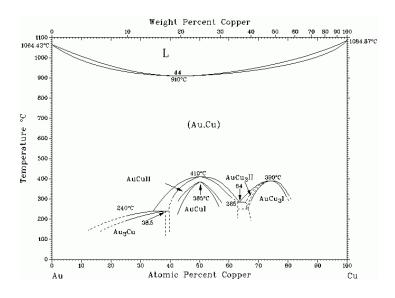
Figure 4 Au-Cu binary alloy phase diagram
