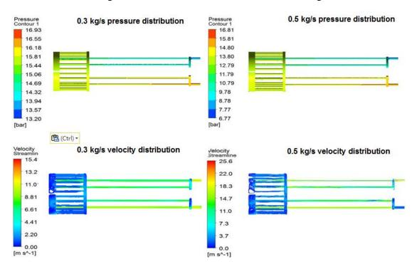
Figure 3-9 Fluid analysis results under mass flow rates of 0.3kg/s and 0.5kg/s
