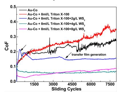
Figure 5-31 Coefficients of friction of Au-Co and Au-Co/WS<sub>2</sub> coatings
