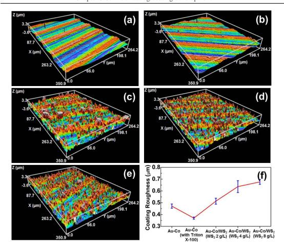
Figure 5-27 3-D surface topography measurements of coatings deposited from different electrolytes: (a). Au-Co, (b). Au-Co with 8 ml/L Triton X-100, (c). Au-Co with 8 ml/L Triton X-100 and 2 g/L WS<sub>2</sub>, (d). Au-Co with 8 ml/L Triton X-100 and 4 g/L WS<sub>2</sub>, (e). Au-Co with 8 ml/L Triton X-100 and 8 g/L WS<sub>2</sub>, (f). Results summary of coating roughness (arithmetic mean height)
