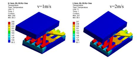
Figure 3-22 Temperature distribution on the RF contact under coiling water velocity of 1 m/s and 2 m/s
