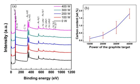
Figure 5-2 XPS spectra (a) and carbon content relation with different sputtering power of the graphite target (b)
