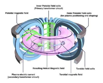
Figure 1-3 Schematic of tokamak [9]
