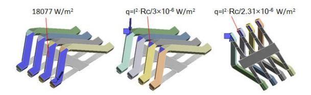
Figure 3-20 Heat fluxes on the louvers
