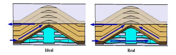
Figure 3-15 Illustration of current flowing in the LA-CUT RF contact during RF tests
