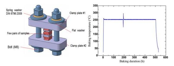
Figure 4-2 Clamping system and baking process of diffusion test
