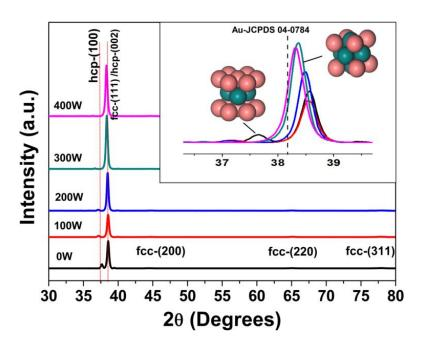
Figure 5-3 XRD patterns of the Au-Ni and Au-Ni/a-C composite coatings
