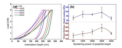
Figure 5-7 Nanoindentation measurement results: (a). Load–displacement curves, (b). Vickers hardness and elastic modulus
