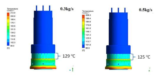
Figure 3-11 Temperature distribution on the RF contact holder
