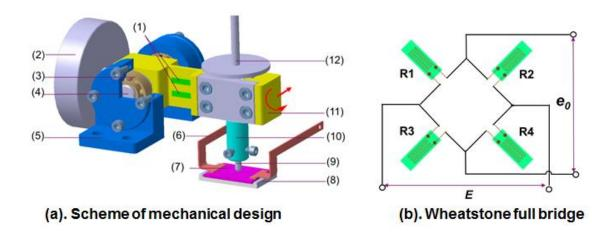
Figure 2-19: (a). Design of the CoF measurement system: (1). Strain gauges (×4); (2). Counterweight; (3). Bearings (×2); (4). Central shaft; (5). Beam support; (6). Electrodes (×2); (7). Plate sample; (8). AlN ceramic plate; (9). Pin sample; (10). Pin sample holder; (11). Cantilever beam; (12). Loading support, (b). Wheatstone full bridge consists of four gauges
