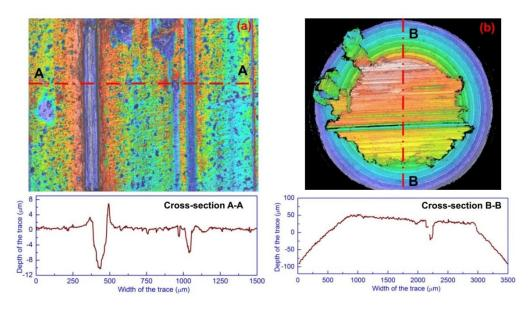
Figure 4-29 3D morphologies and depth profiles of the worn samples: (a) 316L plate sample, (b) CuCrZr pin sample
