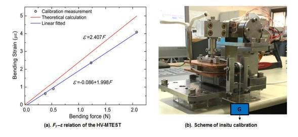
Figure 2-29 Calibration of the HV-MTEST
