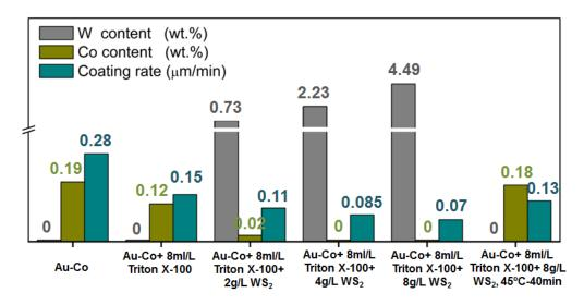
Figure 5-25 W, Co contents and coating rate of different electrolytes under a current density of  $5 \text{ A/dm}^2$
