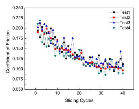
Figure 2-30 Results of CoF during 1-40 cycles [1]
