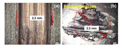
Figure 4-41 Optical microscope images of the worn samples: (a) Rh on CuCrZr plate sample, (b) Ag on CuCrZr pin sample
