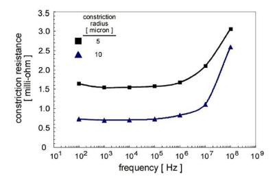
Figure 2-12 Contact resistances under different constriction radii and frequencies [60]
