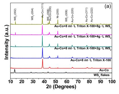
Figure 5-29 XRD patterns of the coatings
