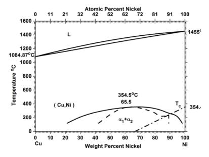
Figure 1 Cu-Ni binary alloy phase diagram
