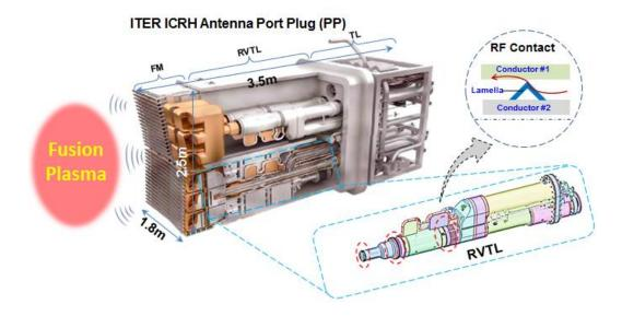
Figure 1-4 Overview of ITER ICRH antenna
