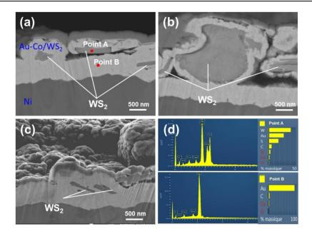
Figure 5-28 Cross-sectional SEM and EDS images of Au-Co/WS<sub>2</sub> coating deposited from electrolyte with 8 g/L WS<sub>2</sub>: (a). SEM image of position 1, (b). SEM image of position 2, (c). SEM image of position 3, (d). EDS point analyses at point A and B positions shown in (a).
