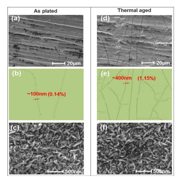
Figure 4-13 Surface morphology of the Rh coating on CuCrZr substrate: (a, d) SEM images of original coating and thermally aged coating (×1,000), (b, e) Cracks on the original coating and thermally aged coating processed by Image J, (c, f) SEM images of original coating and thermally aged coating (×50,000)
