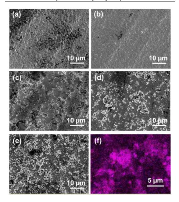
Figure 5-26 SEM and EDS images of the electroplated coatings from different electrolytes: (a). Au-Co, (b). Au-Co with 8 ml/L Triton X-100, (c). Au-Co with 8 ml/L Triton X-100 and 2g/L WS $_2$ , (d). Au-Co with 8 ml/L Triton X-100 and 4g/L WS $_2$ , (e). Au-Co with 8 ml/L Triton X-100 and 8g/L WS $_2$ , (f). EDS mapping of W element on the Au-Co/WS $_2$  coating from electrolyte with 8g/L WS $_2$
