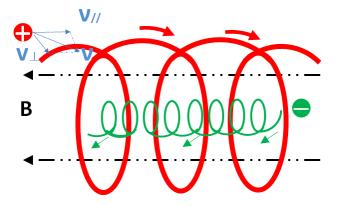
Figure 1-2 Diagram of ions and electrons trajectories in a DC magnetic field
