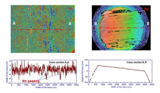
Figure 4-32 3D morphologies and depth profiles of the worn samples: (a) Rh on 316L plate sample, (b) Au-Ni on CuCrZr pin sample
