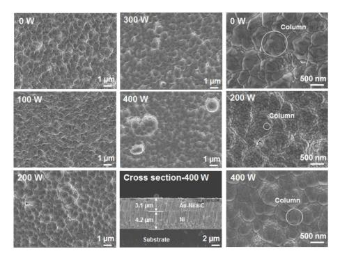
Figure 5-1 SEM images of the Au-Ni and Au-Ni/a-C coatings
