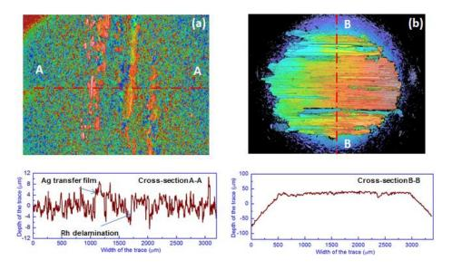
Figure 4-39 3D morphologies and depth profiles of the worn samples: (a) Rh on 316L plate sample, (b) Ag on CuCrZr pin sample
