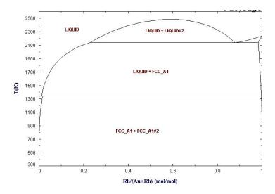
Figure 6 Rh-Au binary alloy phase diagram
