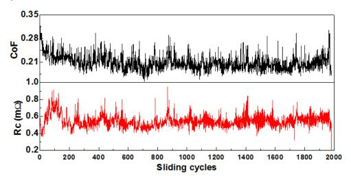
Figure 4-38 Evolution of the Rc and CoF for the Ag on CuCrZr/Rh on 316L pair under 2000 cycles of sliding test at Fn=18 N, 1 mm/s, 200°C, 1.9×10<sup>-3</sup> Pa
