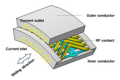
Figure 3-2 Schematic of LA-CUT sliding contact assembly
