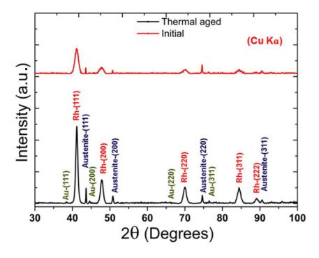
Figure 4-20 XRD patterns of Rh coatings on 316L substrates (original and thermally aged)
