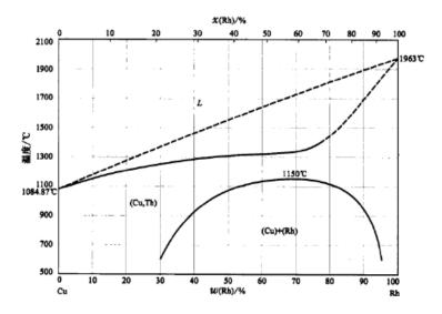
Figure 5 Rh-Cu binary alloy phase diagram
