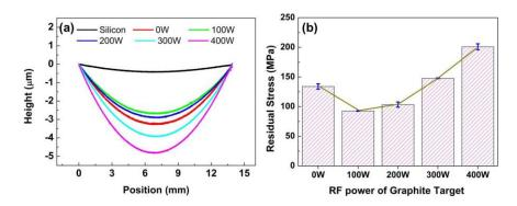
Figure 5-6 Results of coating residual stress measurement on Si (100) wafer: (a). The curvature of Si substrates, (b). Residual stresses of Au-Ni/a-C under different graphite sputtering powers
