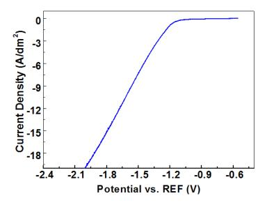
Figure 5-13 Polarization curve for the Ni sulfamate electrolyte
