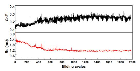
Figure 4-28 Evolution of the Rc and CoF for the CuCrZr/ 316L pair under 2000 cycles of sliding test at Fn=18 N, 1 mm/s, 200 °C, 7×10<sup>-4</sup> Pa
