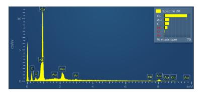
Figure 2: EDS result of top layer
