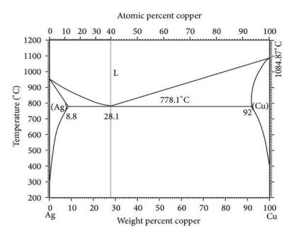
Figure 8 Cu-Ag binary alloy phase diagram
