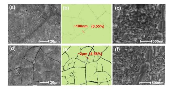
Figure 4-19 Surface morphology of the Rh coating on 316L substrate: (a, d) SEM images of original coating and thermally aged coating (×1,000), (b, e) Cracks on the original coating and thermally aged coating processed by Image J, (c, f) SEM images of original coating and thermally aged coating (×50,000)
