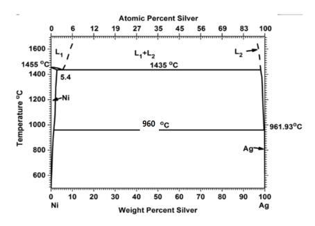
Figure 2 Ag-Ni binary alloy phase diagram
