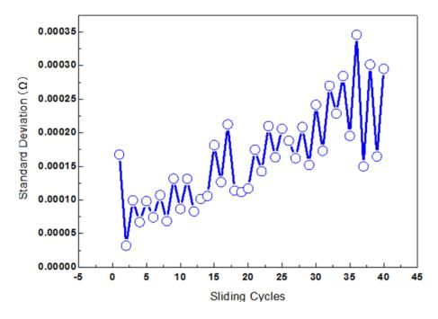
Figure 2-33 Standard deviation of Rc during 1-40 cycles
