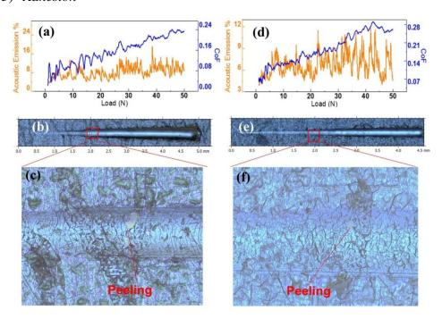
Figure 4-22 Scratch tests results of Rh coating on 316L substrates: (a, d) Acoustic emission and CoF signals of original and thermally aged samples, (b, e) Optical microscope images of scratch tracks of original and thermally aged samples, (c, f) SEM micrographs of cracks on the scratch tracks of original and thermally aged samples
