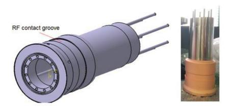
Figure 3-6 RF contact holder design
