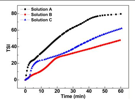
Figure 5-21 Changes of TSI of different electrolytes over time
