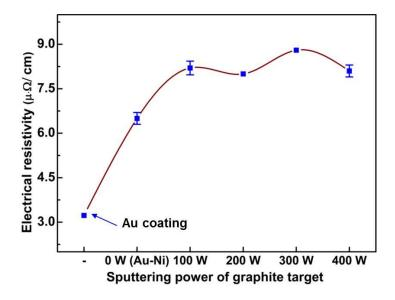
Figure 5-9 Electrical resistivities of Au-Ni and Au-Ni/a-C coatings
