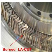
Figure 1-6 Multi-Contact LA-CUT RF contact before and after RF tests<sup>1</sup>
