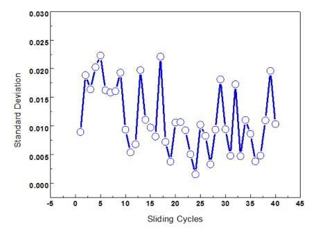
Figure 2-31 Standard deviation of CoF during 1-40 cycles
