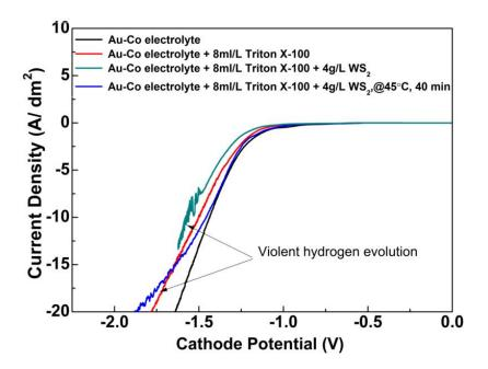
Figure 5-22 Cathodic polarization curves from different electrolytes
