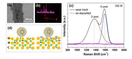
Figure 5-11 Wear track characterizations of 100 W Au-Ni/a-C coating: (a). SEM image of wear track, (b). EDS mapping of C in the position of (a), (c). Raman spectra in the wear track, (d).
