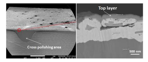
Figure 1: Cross-polishing area and top layer on the coating
