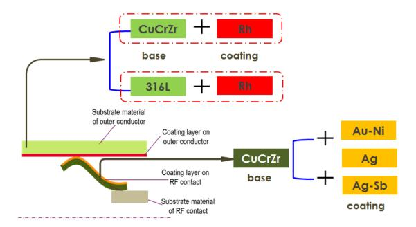
Figure 4-1 Overview of material selection for coating characterizations
