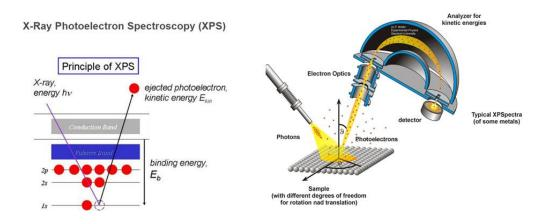
Figure 2-8 Schematic diagram of XPS principle and system [54]
