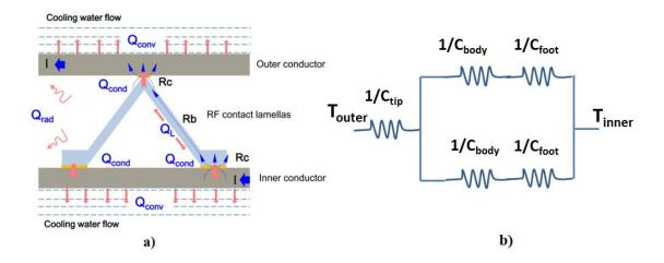
Figure 3-18 Sketch of the ITER RF contact analysis model: (a). thermal-hydraulic model. (b). heat transfer network diagram one RF contact louver
