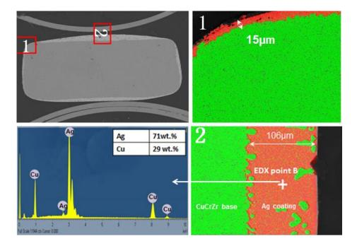
Figure 3-17 SEM/EDS analysis of a damaged CuCrZr louver after RF test
