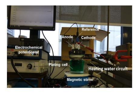
Figure 5-12 Photo of electrodeposition setup
