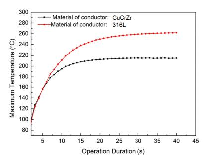
Figure 3-23 Transient temperature on the RF contact with different RF conductor base materials (Rc=7 m $\Omega$ , v=0.5 m/s)
