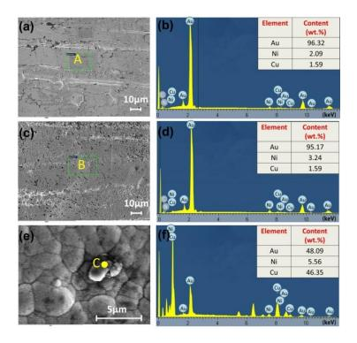
Figure 4-8 SEM/EDS analyses of Au-Ni coating: (a, c, e) SEM images of surfaces of original Au-Ni coating, thermally aged Au-Ni coating (×1000) and thermally aged Au-Ni coating (×8000), respectively; (b, d, f) EDS spectra of area A, area B and point C in, respectively
