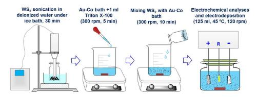
Figure 5-18 Sketch of Au-Co/WS<sub>2</sub> electrolyte preparing flow
