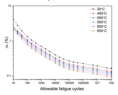
Figure 2-25 Allowable fatigue cycles (N) for 304 type stainless steel [102]
