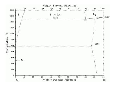
Figure 7 Rh-Ag binary alloy phase diagram
