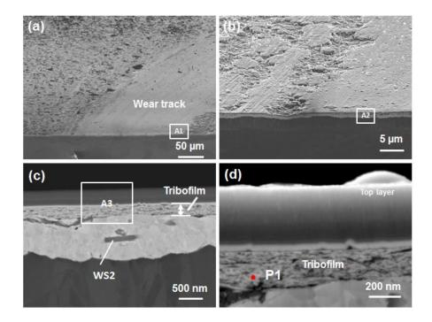
Figure 5-34 SEM images in the wear track of Au-Co/WS<sub>2</sub> (from electrolyte with 8g/L WS<sub>2</sub>): (a). Overview of wear track, (b, c, d). Detail views in the area of A1, A2 and A3. (There is a 300 nm thick top layer observed, which is generated during the cross-sectional sample preparation by using cross-polisher. The provement is shown in Appendix C.)
