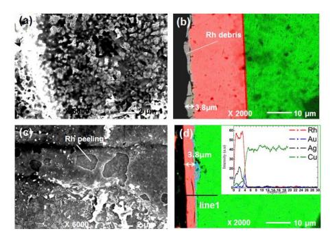
Figure 4-26 SEM and EDS mapping of Ag-Sb (on CuCrZr) and Rh (on CuCrZr): (a) SEM image of Ag-Sb surface, (b) EDS mapping of Ag-Sb cross-sectional surface, (c) SEM image of Rh surface, (d) EDS mapping of Rh cross-sectional surface
