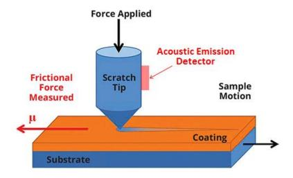
Figure 2-5 Schematic diagram of scratch test [43]
