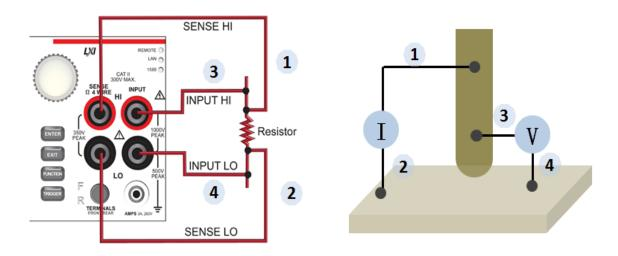
Figure 2-20 Keithley DMM7510 71/2 four wire connection for the Rc measurement
