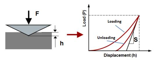
Figure 2-6 Schematic diagram of the nanoindentation test and typical P-h curves
