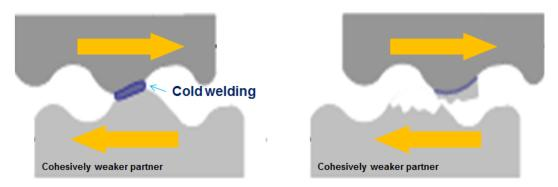
Figure 2-13 Illustration of adhesive wear [69]
