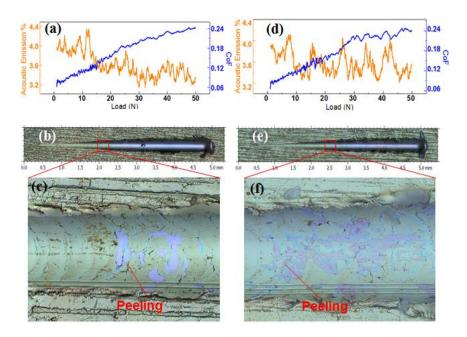
Figure 4-9 Scratch tests results of Au-Ni coating on CuCrZr substrates: (a, d) Acoustic emission and CoF signals of original and thermally aged samples, (b, e) Optical microscope images of scratch tracks of original and thermally aged samples, (c, f) SEM micrographs of cracks on the scratch tracks of original and thermally aged samples
