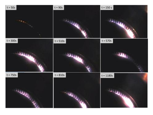
Figure 3-14 Status of the LA-CUT RF contact during 1.2 kA, 1200s operation
