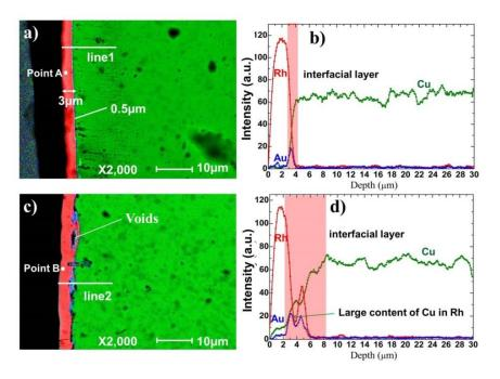
Figure 4-17 Mapping and depth profile of the Rh coating on CuCrZr substrate: (a) EDS mapping of original sample section, (b) Elements profiles along line1, (c) EDS mapping of thermally aged sample section, (d). Elements profiles along line2
