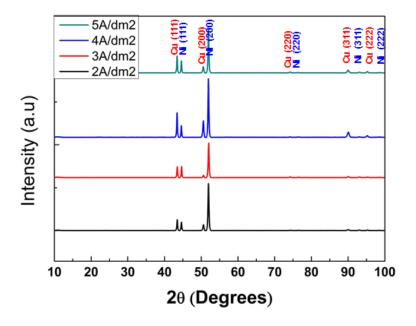
Figure 5-15 XRD patterns of the Ni coatings
