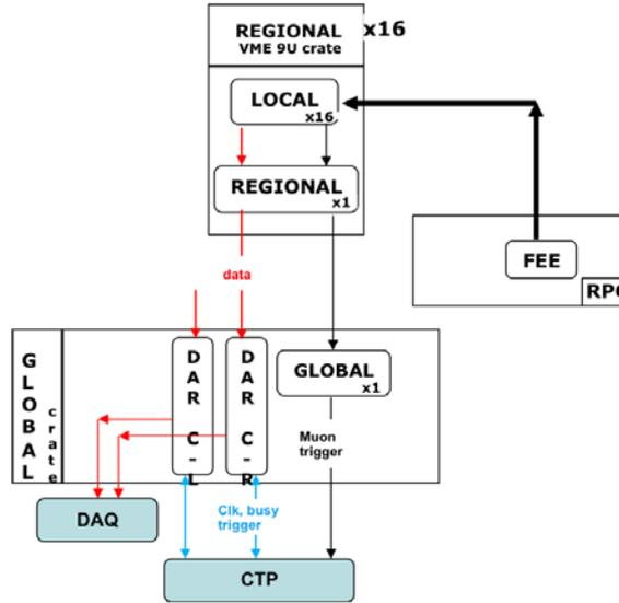
Figure 4.7: Schematic of the MTR readout electronics architecture.
