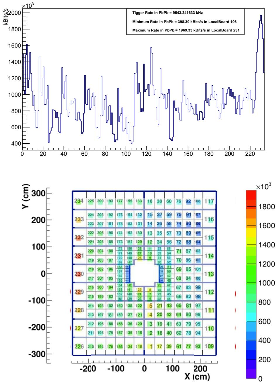
Figure 4.11: Data flow per local board for the Pb-Pb run 246036 (top). 2D-view of the data flow per local board (bottom).
