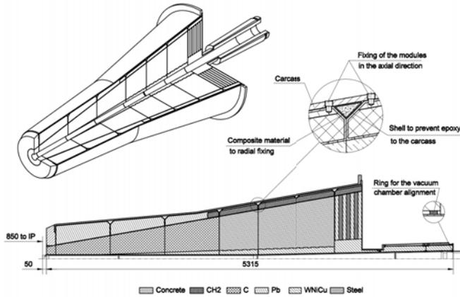
Figure 2.7: Layout of the front absorber [194].
