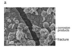
Fig. 1. (a) secondary eletron (SE) image of the thin corrosion surface and (b) Backscatered electron (BSE) and Energy dispersive chemical maps of the cross section of thin corrosion layers.
