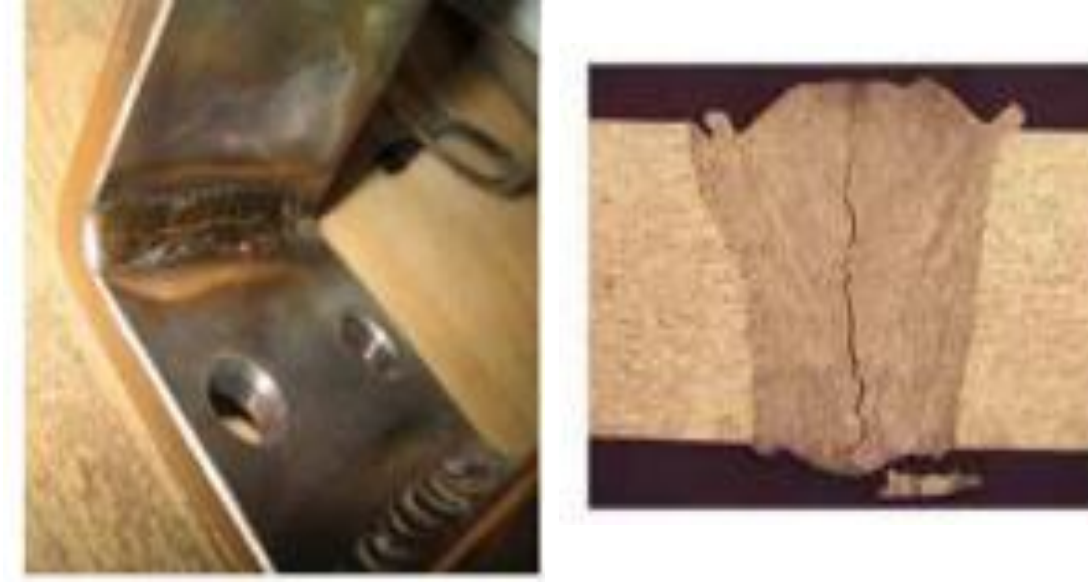
Hot cracking in welding
