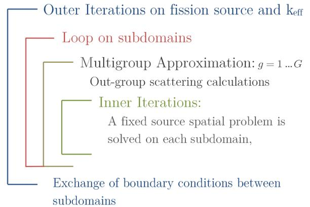
Figure 2: Domain Decomposition algorithm using multigroup Jacobi iterations
