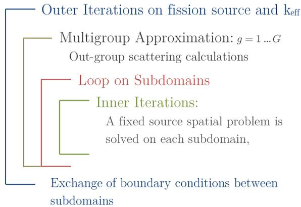
Figure 1: Domain Decomposition algorithm using one-group Jacobi iterations
