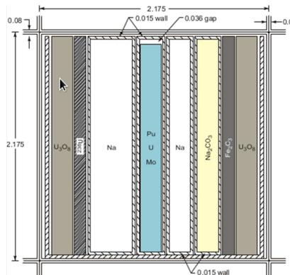
**Figure 5.** Typical ZPPR-10A Single Column Fuel Unit Cell
