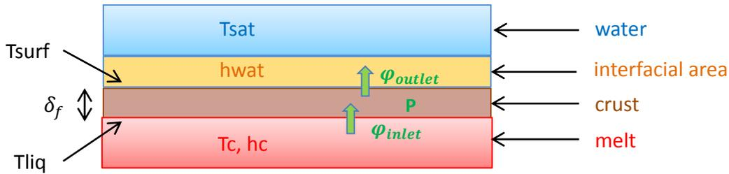
Fig. 2 Heat fluxes at the interface corium/water with crust.
