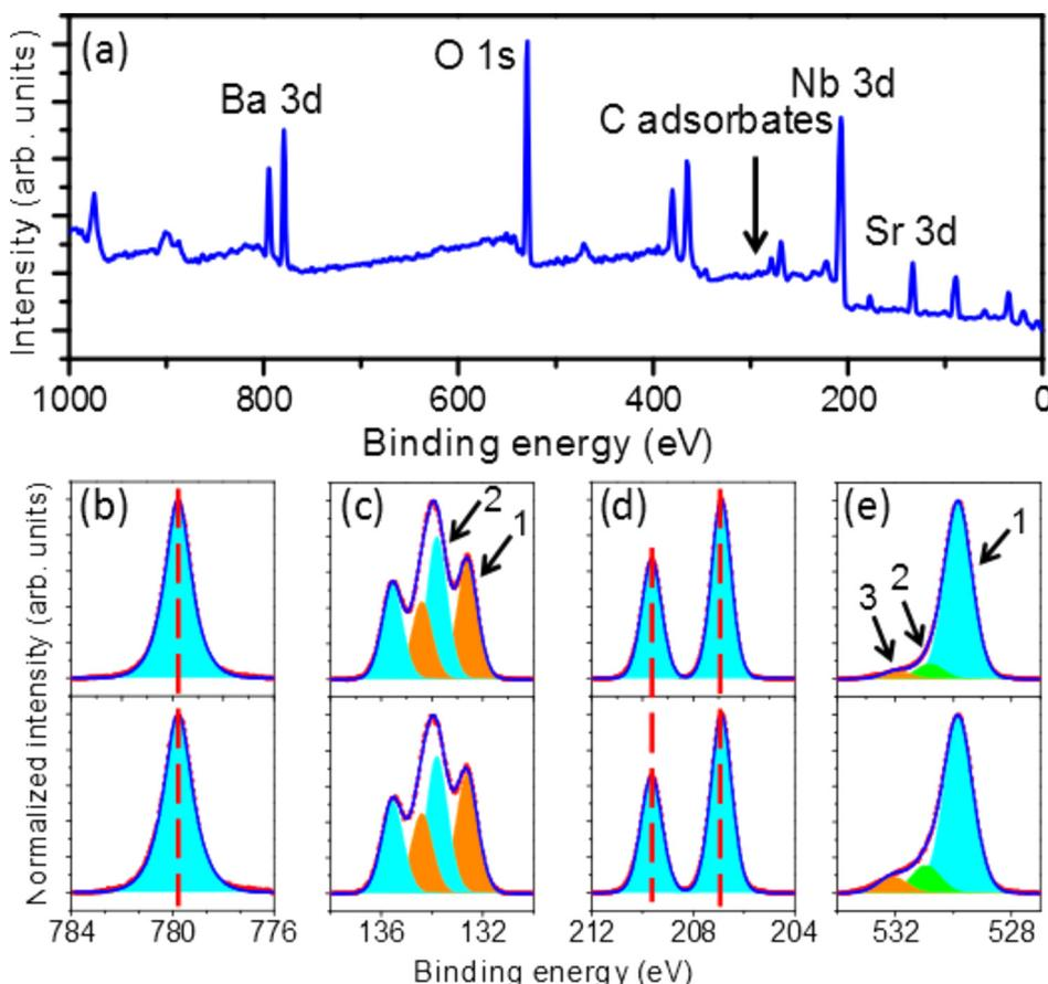
FIG. 4. (a) XPS survey spectrum of SBN(001) single crystal. Core level spectra: (b) Ba 3d<sub>5/2</sub>; (c) Sr 3d; (d) Nb 3d; (e) O 1s core level spectra at normal (top) and 60° (bottom) emission angles.
