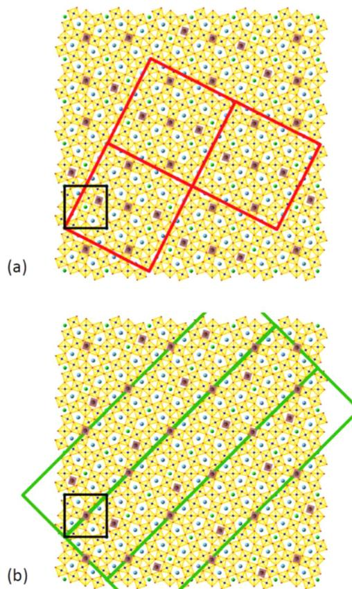
FIG. 3. Schematics of the  $(\sqrt{5} \times \sqrt{5})R26.6^\circ$  (a) and  $(5\sqrt{2} \times \sqrt{2})R45^\circ$  (b) reconstructions due to different cation vacancy distributions. Three unit cells are shown for each reconstruction. The bulk cation vacancy concentration of 1/6 is respected as are the A1/A2 site ratios in the reconstructed unit cells. Vacancy sites are indicated by the small shaded squares. The SBN ( $1 \times 1$ ) unit cell is the small (black) square.
