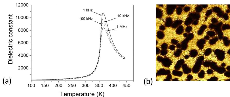
FIG. 1. (a) Dielectric response of SBN single crystal for frequencies between 1 kHz and 1 MHz. The Curie temperature is 360 K. (b) PFM phase response of SBN surface. Phase scale:  $180^\circ$  from black to white.
