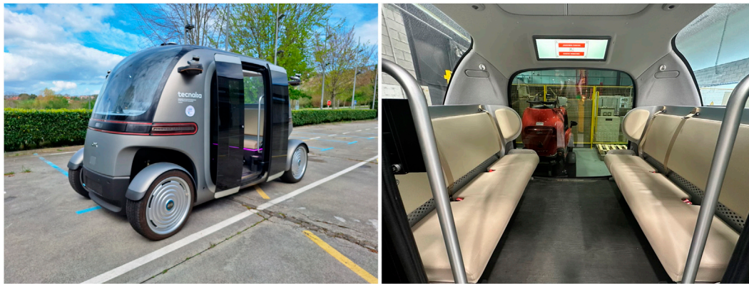
FIGURE 1 Pixis Robobus, an autonomous shuttle used in the real-world simulated user study (left) and interior design with HMI (right).
