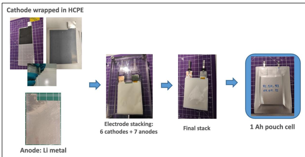
Figure S1. 1 Ah pouch cells assembling process.
