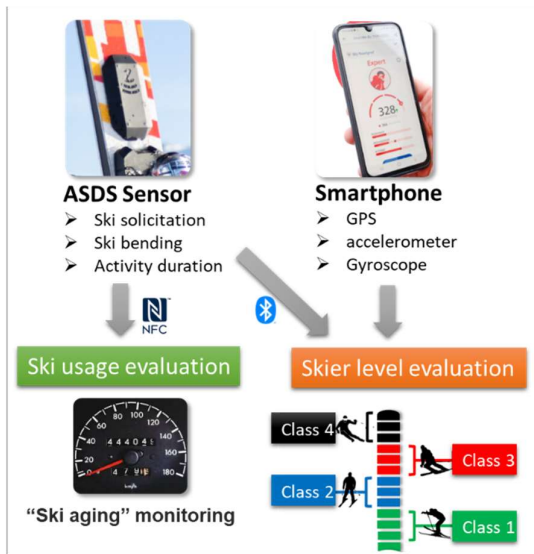
Fig. 4. Illustration of the operating principle of two key insights derived from the Autonomous Ski Deflection Sensor (ASDS) system: ski usage/aging evaluation and skiing level classification
