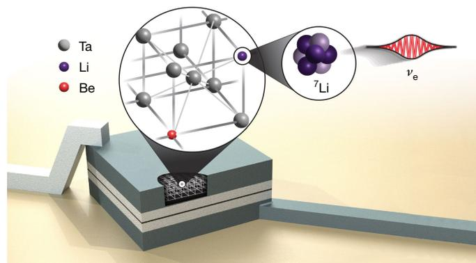
**Fig. 1 | <sup>7</sup>Be EC in an STJ.** Schematic of the STJ sensor showing the five layers described in the text. The <sup>7</sup>Be radioactive source is sparsely implanted into the Ta lattice of the absorber layer. The zoomed-in image (top right) shows the final state after EC decay including <sup>7</sup>Li recoil and  $\nu_e$ .
