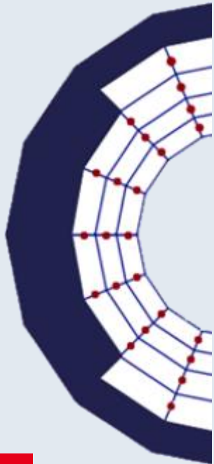
A_{\parallel} and j_{\parallel} are defined on a poloidally and toroidally staggered grid
