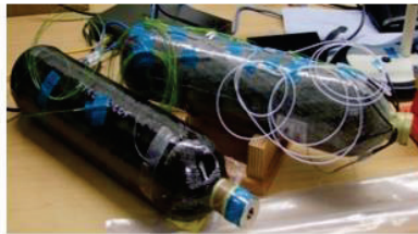
Composite tanks with embedded optical fiber sensors
