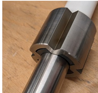
Figure 3: Positioning the ferrite inserts in the foliage of the quadrifoil plates
