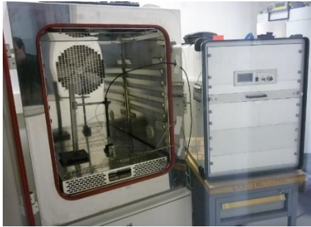
😊 Test in climatic chamber (CEA) [80% RH, 15° – 85°C]
