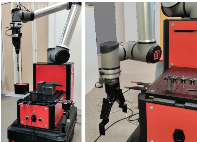
Figure 1: Display of the OSCAR platform equipped with a tool changer allowing the use of a screwdriver (left) or gripper (right).
