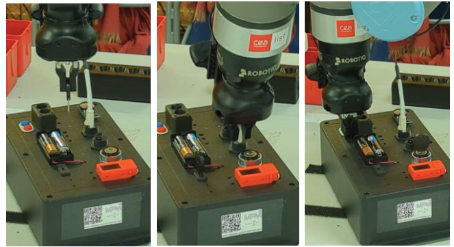
Figure 9: Illustration of the system performing the defined tasks: inserting the key (left), grasping the Ethernet cable (centre) and pushing the red button (right).
