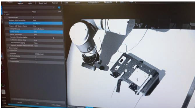
Figure 5: Illustration of a Photoneo scan used to locate objects whose CAD models are known.
