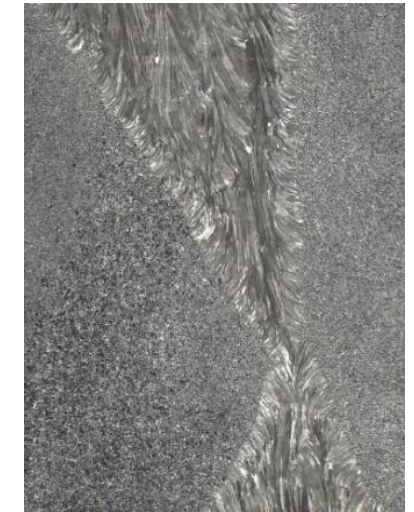
Weld microstructure (EDF)
