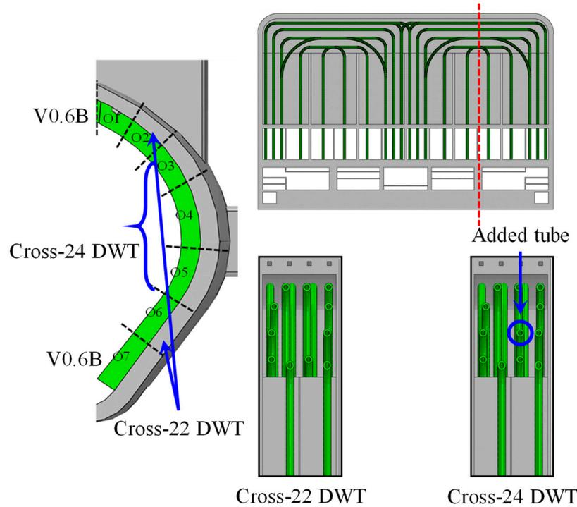
Figure 9. New DWT layout and COB poloidal distribution.
