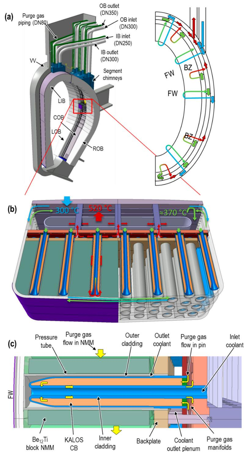
**Figure 16.** Overview of the HCPB “pin” BB design layout: (a) view of a HCPB DEMO sector with segments and feeding pipes (left) and flow scheme in a segment (right); (b) radial–toroidal section view of a COB segment; (c) close-up view of a radial–toroidal section of a fuel-breeder pin.
