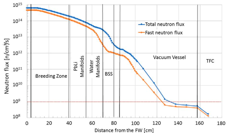
**Figure 4.** Inboard radial profile of the total (blue) and fast (red) neutron flux at the equatorial plane.
