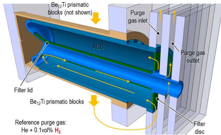
Figure 17. Detail of the purge gas flow.
