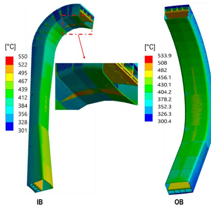
**Figure 23.** Global thermal analysis of an IB segment (left) and COB segment (right).
