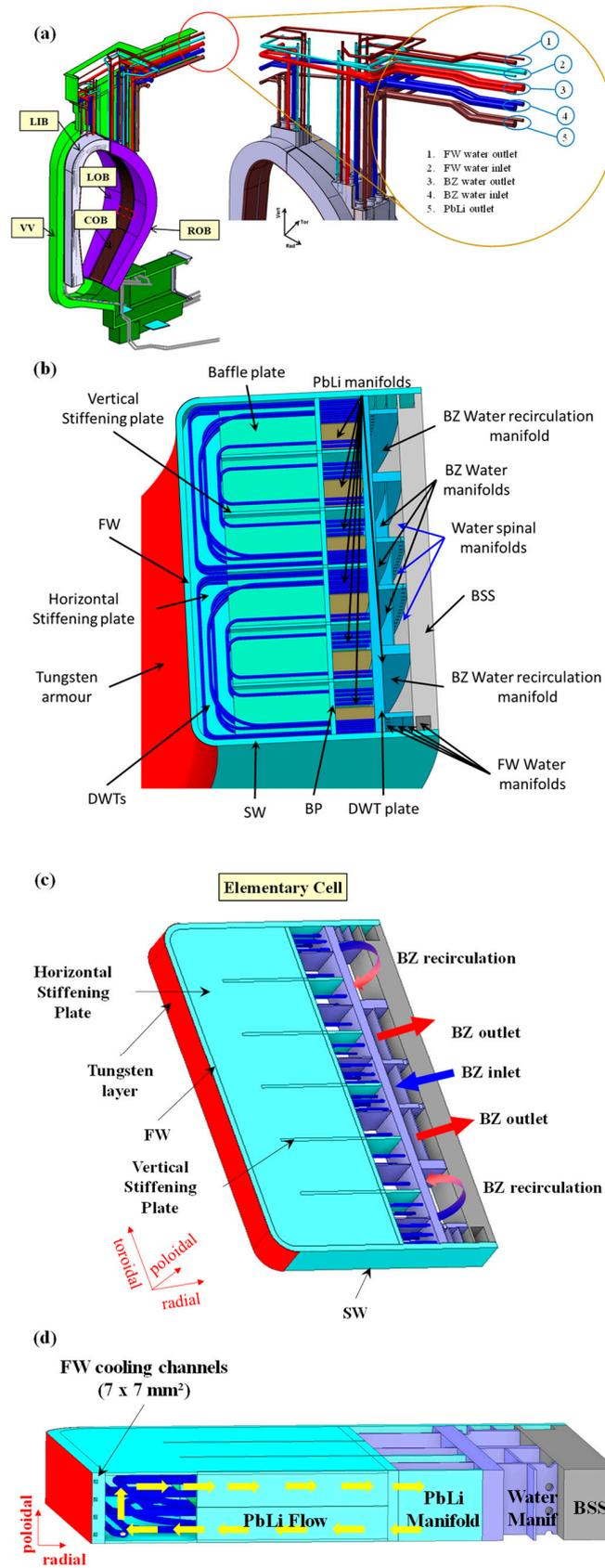
**Figure 2.** Overview of the WCLL “DWT” BB design layout: (a) view of a WCLL DEMO sector with segments and feeding pipes; (b) radial–toroidal section view of a COB segment; (c) WCLL elementary cell; (d) radial–poloidal cross section view of a WCLL elementary cell.
