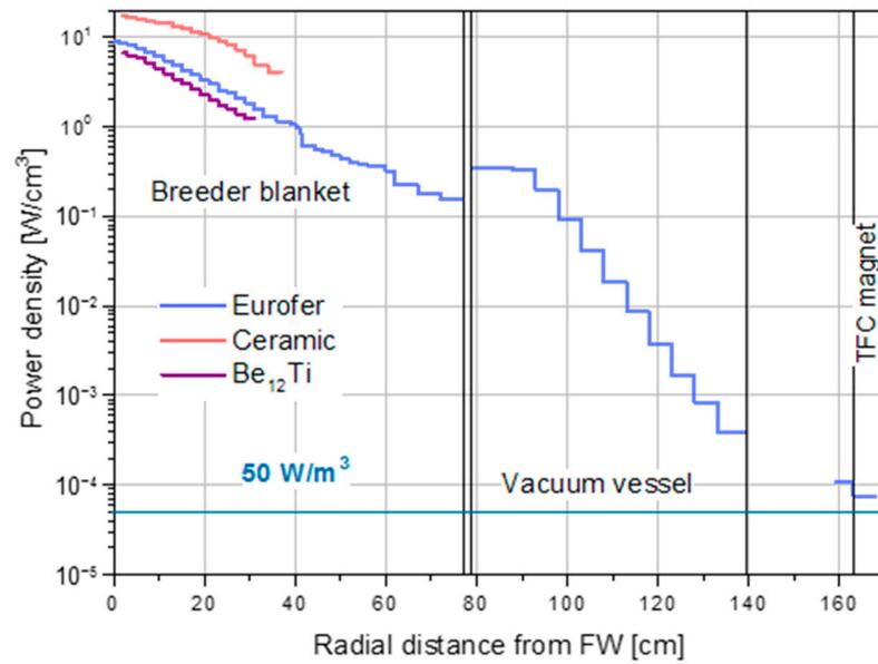
Figure 19. Power density as function of the radial coordinate in an inboard segment.
