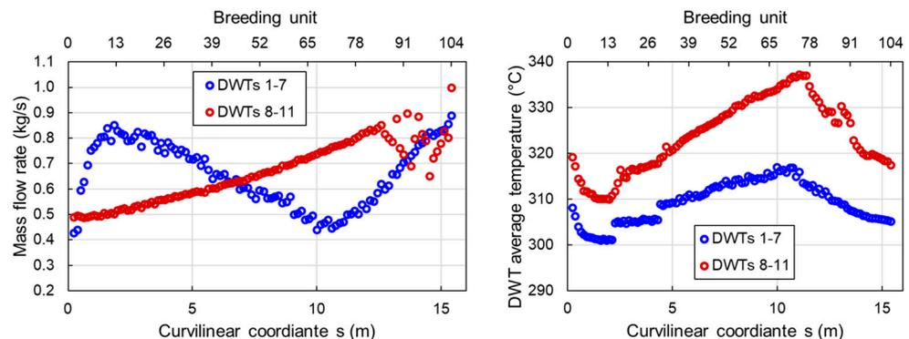
Figure 10. COB mass flow rate and temperature distributions.
