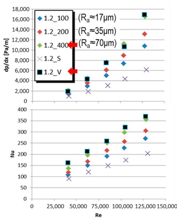
Figure 26. Parametric thermal-hydraulic analyses in a FW under a total heat flux peak of 1.2 MW/m<sup>2</sup> showing pressure drop per unit length (top) and Nu number (bottom) as function of Re for different FW channel turbulence promoter configurations with sand roughness  $R_a$  of 17  $\mu\text{m}$  (labeled as “1.2\_100”), 35  $\mu\text{m}$  (labeled as “1.2\_200”) and 70  $\mu\text{m}$  (labeled as “1.2\_400”), smooth channel (labeled as “1.2\_S”) and V-ribs (labeled as “1.2\_V”).
