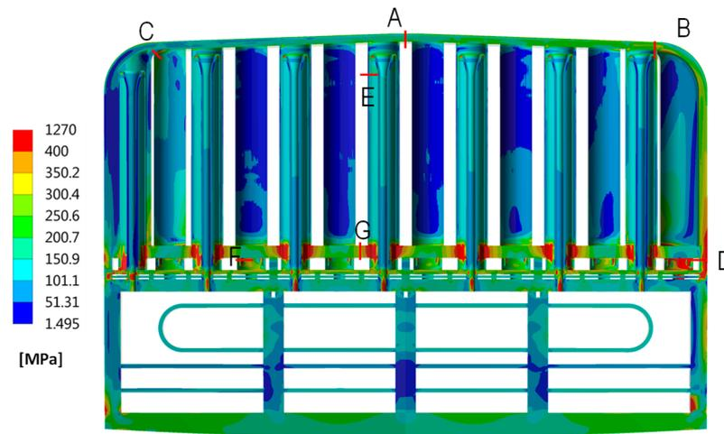
**Figure 27.** Von Mises stress distribution of primary and secondary loads in the equatorial midplane of a COB segment in normal operation. Letters A to G refers to the paths used for the stress linearization.
