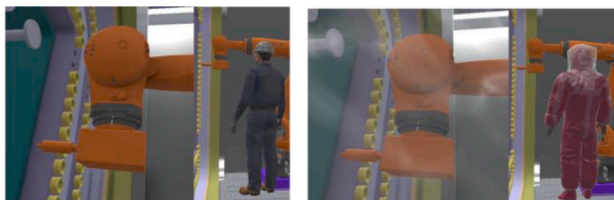
Fig. 11. Simulated visual field with avatar in a standard suit and simulated visual field with avatar in ventilated suits.
