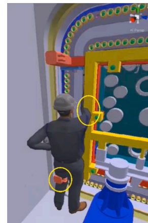
Fig. 12. Accessibility study to the bolts with clashes detection.
