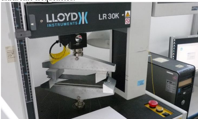
Figure 2: FOUR-POINTS BENDING TEST SETUP
