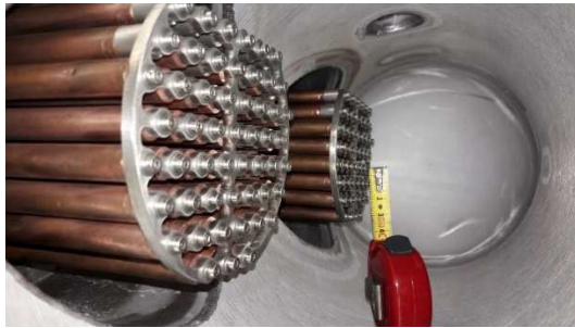
Figure 2 - Vertical and horizontal multi tube heat exchangers for superfluid helium cooling and corresponding heat transfer and temperature profiles: (a) in turbulence studies [3] at CEA-Grenoble test facility (tube dimensions D42xL400 mm.mm) and (b) in D2 magnets [4] for HL-LHC (tube dimensions D10xL500 mm.mm)
