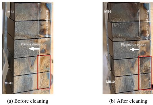
Fig. 7. Visual comparison before and after cleaning by the adhesive tape. (For interpretation of the references to color in this figure legend, the reader is referred to the web version of this article.)
