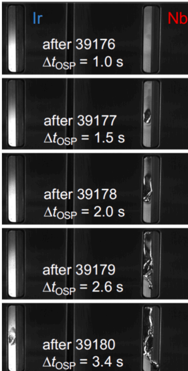
Fig. 2. High resolution images of the Ir and Nb samples after each of the four consecutive exposures of increasing duration ELMI H-mode in the AUG outer divertor. The sample length is 39 mm, for 3D geometry refer to Fig. 3. The duration of steady outer strike point \Delta t_{OSP} is indicated in the images — the overall exposure is longer, see Sec.2.3.2 for details.
