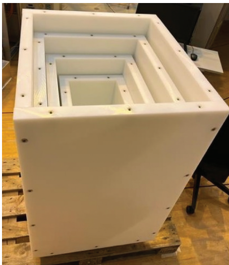
Fig. 7. Photograph of the four innermost PE boxes (without their lids) used for experimental measurements of neutron and gamma-ray dose attenuation.
