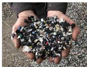
Figure 1: SRF: a blend of paper, card, wood, textiles and plastic (LHV: 18 -25 MJ/kg)
