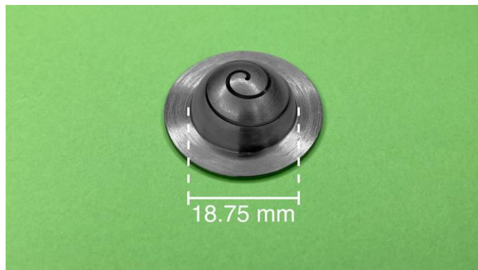
Fig. 1. Picture of the 3D coded mask.
