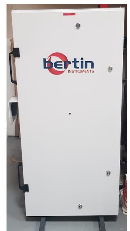
Figure 1. A Saphygate G Radio portal Monitor used in laboratory environment for the ENTRANCE project
