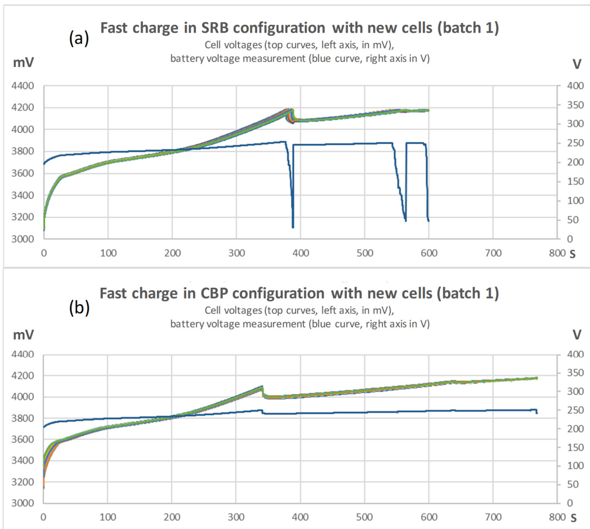
Figure 15. Comparison of charge for CBP and SRB configurations using cells from batch 1: (a) SRB configuration results; (b) CBP configuration results. Cell voltages colors only to improve contrast.
