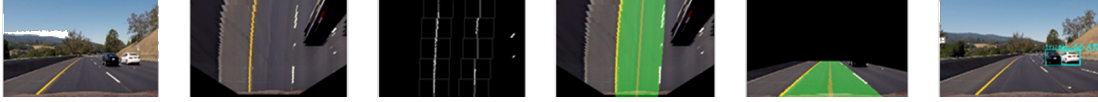
Fig. 2. ADAS vision processing stages: front view (ImgSrc output), bird-eye view (PerspWarp output), lane detection (2 stages), inverse perspective (PerspUnwarp output), and object detection.
