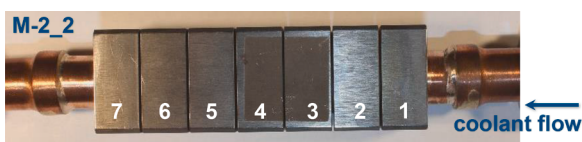
Fig. 1.. Top view image of component M-2_2; exposure area on block 3 and 4 correspond to loading in the e-beam facility EMS-60 at 10 \text{ MW/m}^2 .
