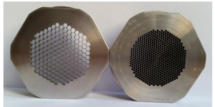
Fig. 8. Stainless steel collimator grids prepared by electrical discharge machining. In the grid on the left, the cells have an apothem of 2 mm and in the grid on the right, the apothem is 1 mm.
