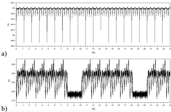
Fig. 4 24h-grid profiles a) frequency, b) voltage
