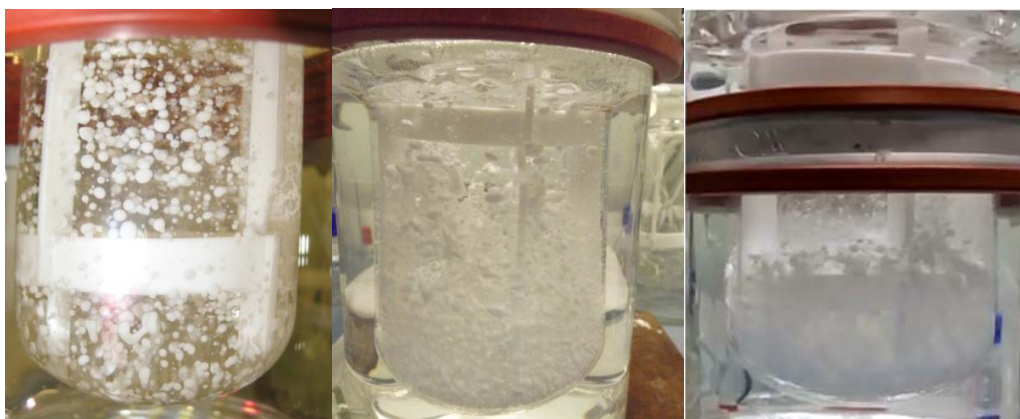
Fig. 3. Batch experiments of BSN precipitation in emulsion. Effect of the droplet volume fraction, from left to right: 2%, 10% and 16%.
