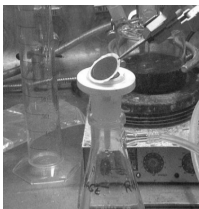
FIG. 3. Dissolution residues on a Millipore® filter.
