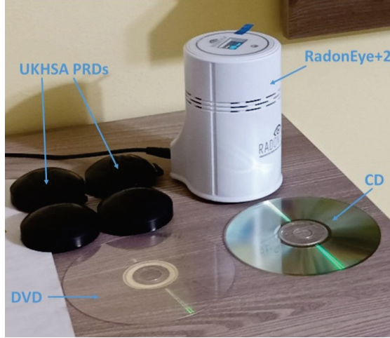
Figure 1: Typical placement of the detectors used in the campaign
