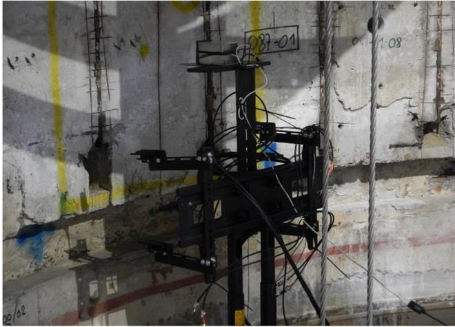
Fig. 6. Gamma spectrometry equipment at position.
