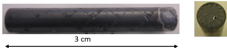
Figure 4: Sample N°1 brazed with the reference BraSiC ® alloy.
