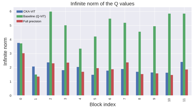
Fig. 4: Infinite norm ( \|\mathbf{x}\|_\infty = \max_i |x_i| ) of the values of the query matrix, comparing the CKA-ViT (blue), the baseline correlation used in the Q-ViT approach (in green) and the full precision model (in red).
