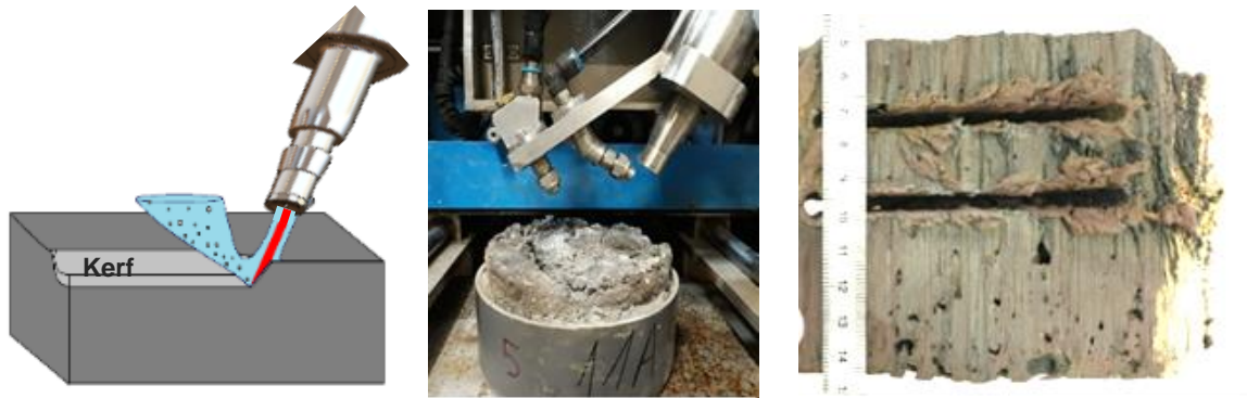
Figure 5: Laser deep gouging of fuel debris [19] Left: sketch of the laser head operation Center: Testing the laser deep gouging of an ex-vessel fuel debris simulant Right: Top view of a fuel debris simulant after 2 kerfs have been gouged
