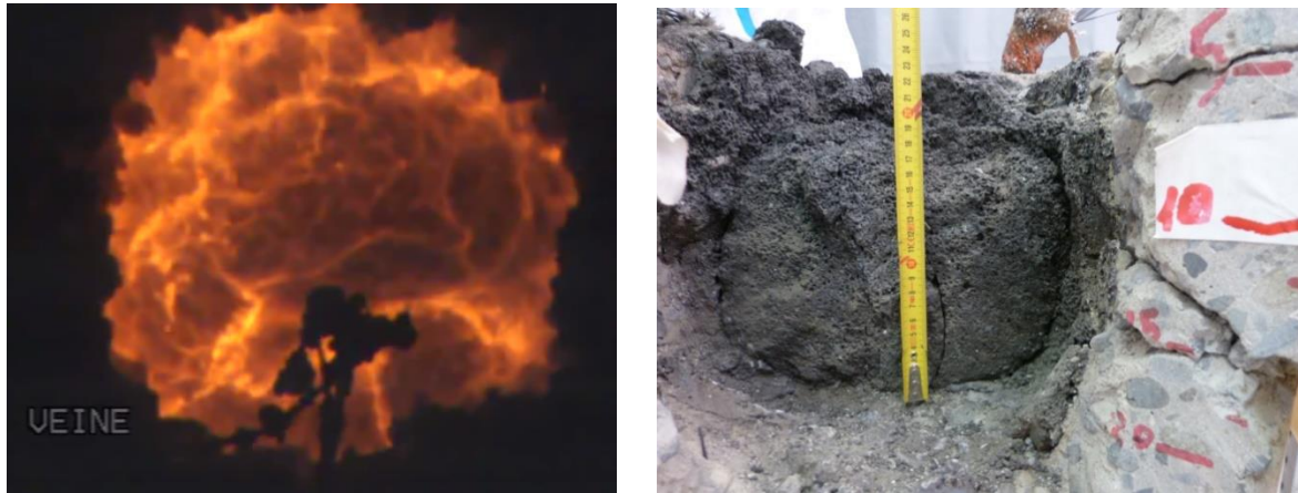
Figure 2: MCCI Test VF-U1 – Left: during MCCI – Right: during fuel debris retrieval
