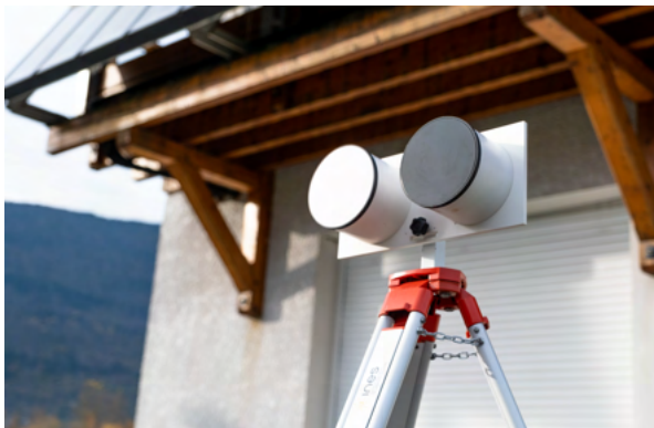
Figure 2: SENS sensor : measurement of the equivalent temperature of a surface (source picture: INES)
