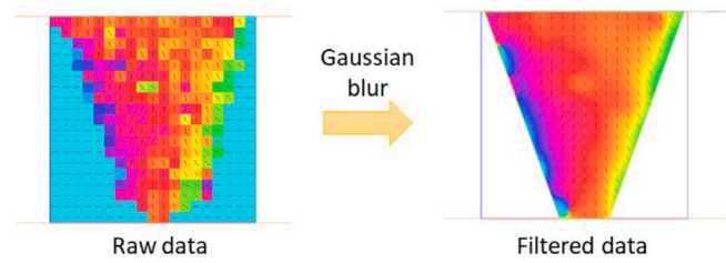
Fig. 2. Example of a Gaussian blur filter applied to raw MINA data to regularize the description inside the welded part (standard deviation 2 mm).
