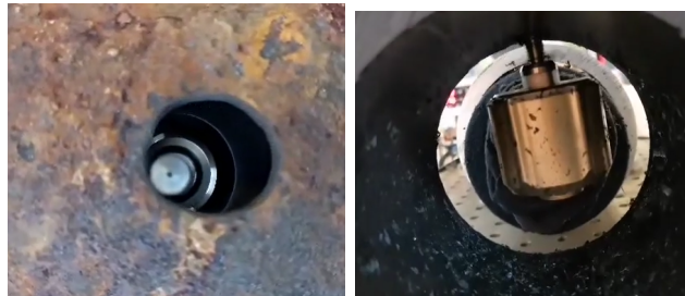
Fig. 10. Machining tests are realized inside the pipe on cast iron (left) and PE (right).
